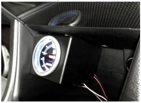
2. Next, plan your wire routing and start to wire the gauge. You can obtain power from a number of locations including behind the radio or in the fuse panel. This guide assumes you have done simple electrical work and you can figure this out on your own (grab a friend if not!). Here is an example of tapping into the WRX fuse box using a fuse tap (not included - sold in stores or Amazon):
