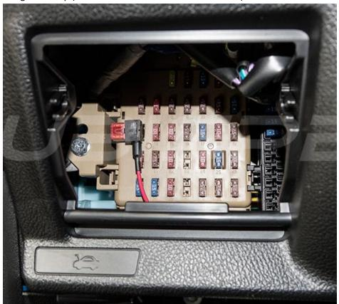
The illumination wire can come from a number of sources as well. The purple wire from the hazard switch or the display switch is one example (you will need to remove the trim around the radio console):
