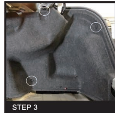
STEP 3 Remove the three plastic clips and pull out the trunk side liner cover to access the back of the tail light
