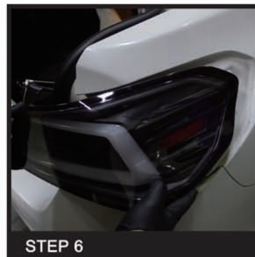
STEP 6 Seat the new tail light assembly in place
