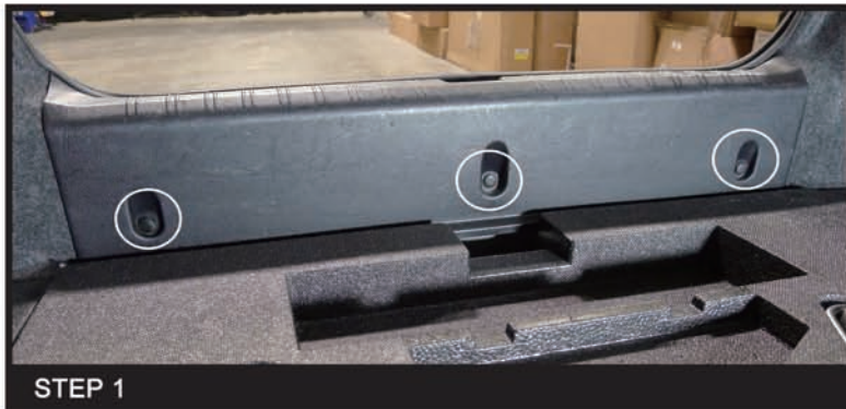
STEP 1 Remove the three plastic clips
