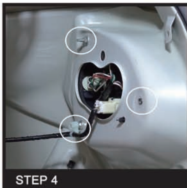
STEP 4 Disconnect the tail light harness and remove the three 8mm tail light mounting nuts
