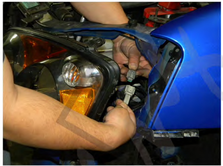
12. Disconnect headlight harness
