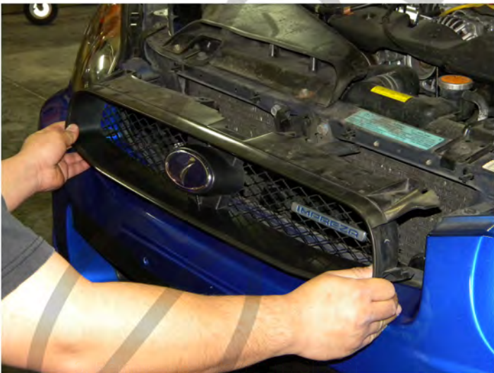
27. Install front grille please repeat picture order from 1 to 27 for opposite side
