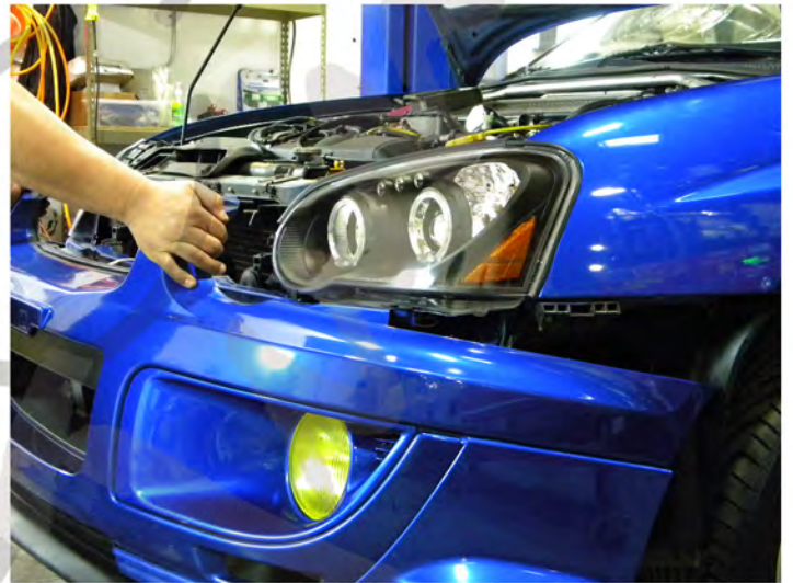
20. Install the front bumper
