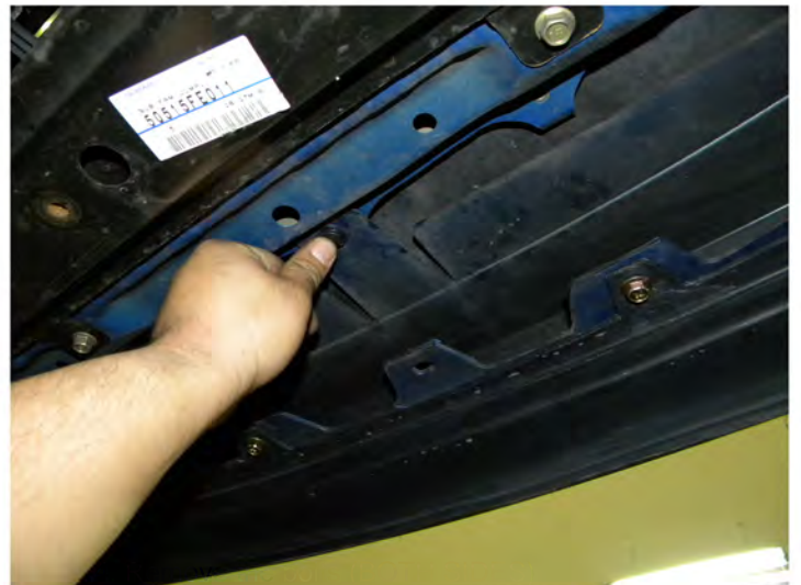
22. Install three clips
