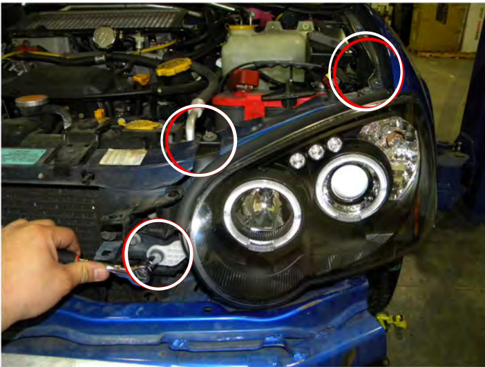
19. Install three 10mm headlight bolts
