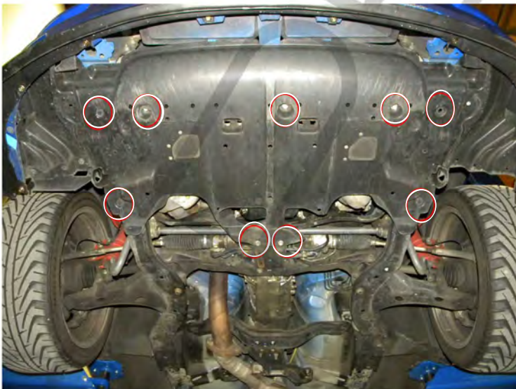
3. Remove five bolts and four clips
