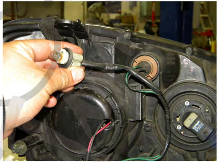
14. Remove driving light harness from OEM headlight
