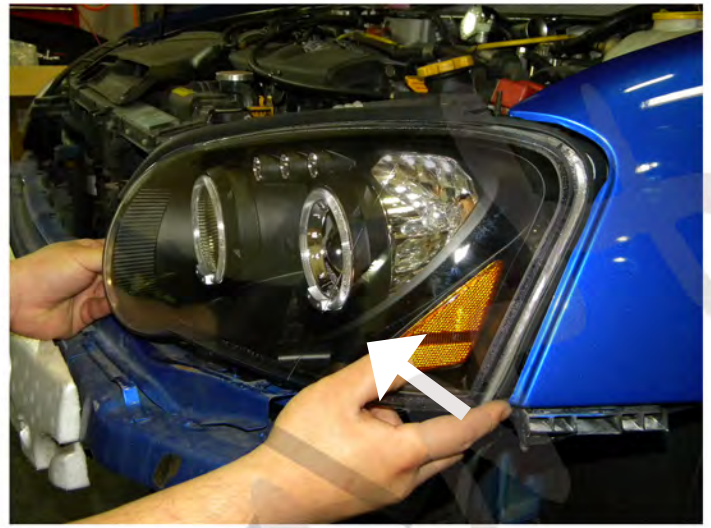
18. Connect headlight harness then install the headlight Please see the "Halo and L.E.D installation instructions" If your headlights don't have HALO or L.E.D. You can skip
