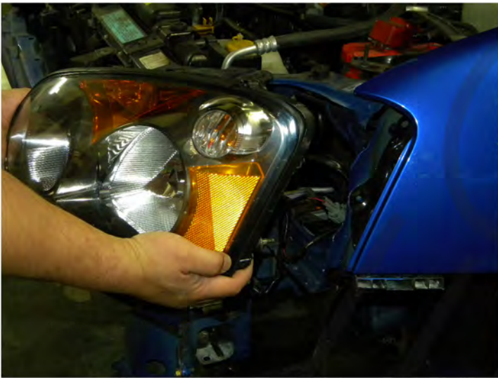
13. Remove the headlight
