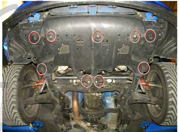
26. Install cover (five 10mm bolts and four clips)
