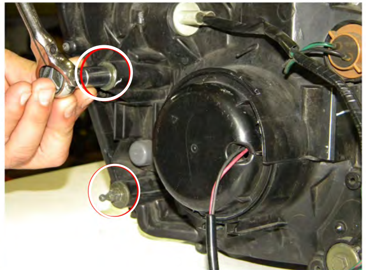
16. Remove two pins from OEM headlight
