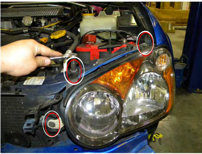
11. Remove three 10mm headlight bolts
