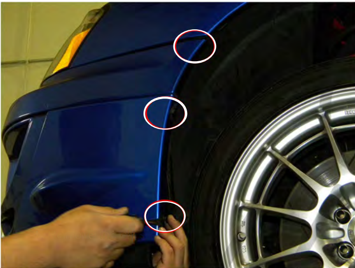
25. Install one 10mm bolt and two clips
