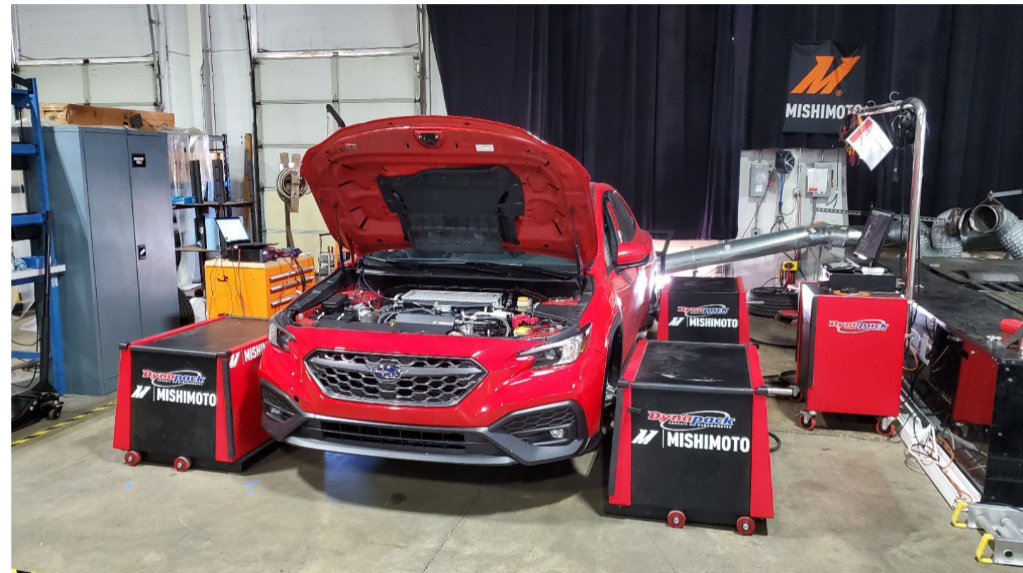
Figure 12: The 2022 Subaru WRX being set up on a Dynapack dynamometer and prepared for testing
