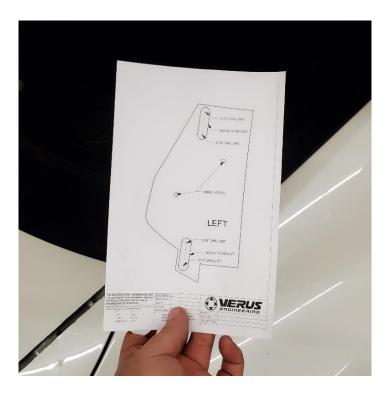
**2.4.** Attach the template to their respective sides by using a couple pieces of tape.
