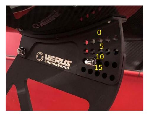
**2.18.** To finish installing the rear wing, we have to install the endplates. We offer both carbon (upgrade) and sheet aluminum (standard). Both install the same. We include aluminum washers for M4 FHCS, and o-rings to reduce marring of the aluminum of carbon fiber. Install the o-ring on the washer, and install into the endplate and rear wing as shown below. Finger tight should be plenty.
