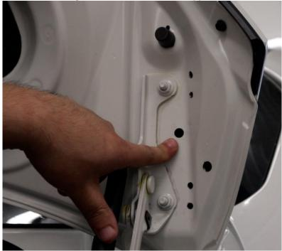
**2.5.5.** To properly install the rivet nut, you will want to thread the rivet nut onto the tool as shown below. Note the rivet nut in the picture below is incorrect for this segment. Use this photo as a visual aide.
