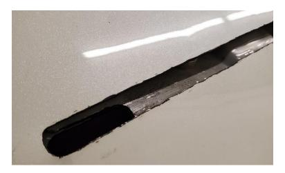
**2.11.** Prepare the beauty plate, and trunk surface with a 50/50 isopropyl alcohol/water mix, and apply one side of the pre-cut double-sided tape. We recommend applying the side with the white backing to the beauty plate.
