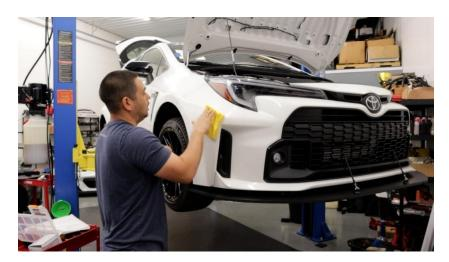
**2.5.** Locate the appropriate template for the side you want to install first. Cut the template out and tape it to the bumper following the guidelines on the template.
