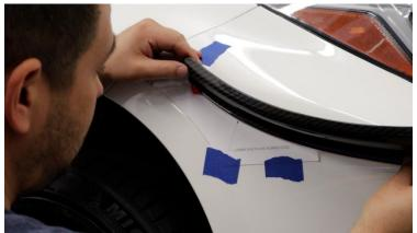
**2.9.** Once you are happy that the placement of the dive plane, begin pulling the red backing off while holding the dive plane in place.
