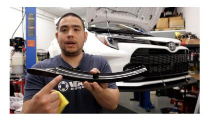
**2.7.** Peel the white backing off and, apply the correct pre-cut VHB tape pieces to the dive planes. Have the red backing facing away from the dive plane.
