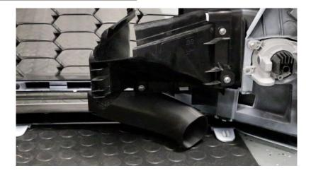
2.6. After the inlet ducts are installed, push the radiator support tray back in place to figure out where you need to trim it.
