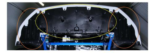
2.5. At this point you should be looking at the back side of the bumper grill. You will need to pull the radiator support tray down slightly to find the screw we need to remove for installing the inlet duct. This screw can be seen below. **Note: This is the right-hand side.**
