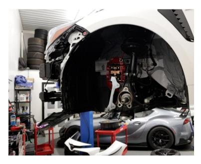
2.12. Now we need to install the backing plate kit. Start by using the hub mounting bolts for locating the backing plate. **Note: The carbon duct should face inward and should be towards the rear of the car as shown below.**
