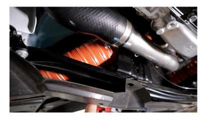
**2.13.3.** Route the hose above the crank pulley and CV axle.
