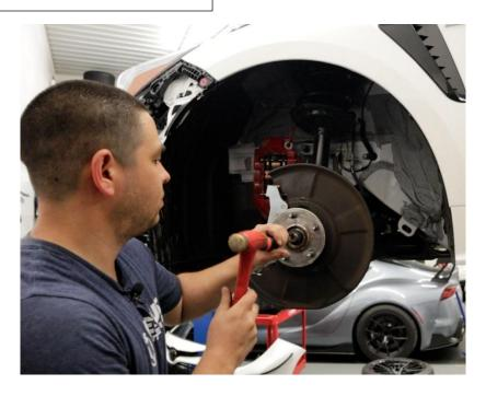
**2.10.1.** After the keyway is opened up, remove the axle nut using the 30mm socket and impact gun.
