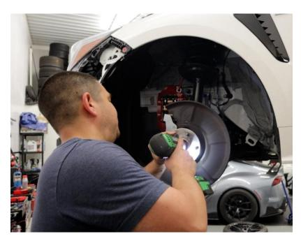
2.11. After the axle nut is removed, we now need to remove the hub assembly. Do so by using a combination of the 19mm wrench and 19mm socket with a 6" extension and swivel adapter.
