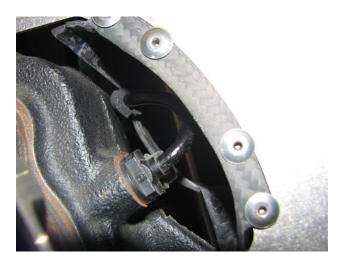
**2.12.4.** After you ensure the speed sensor wire is good and protected, you may now reinstall the hub assembly in reverse order from earlier. Start all three bolts by hand and then torque to factory spec.
