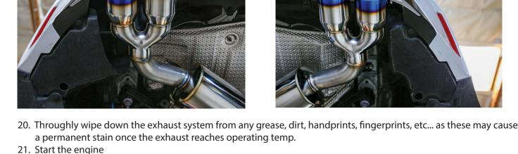
22. Check for any leaks, fitment issues, rubbing, etc..
