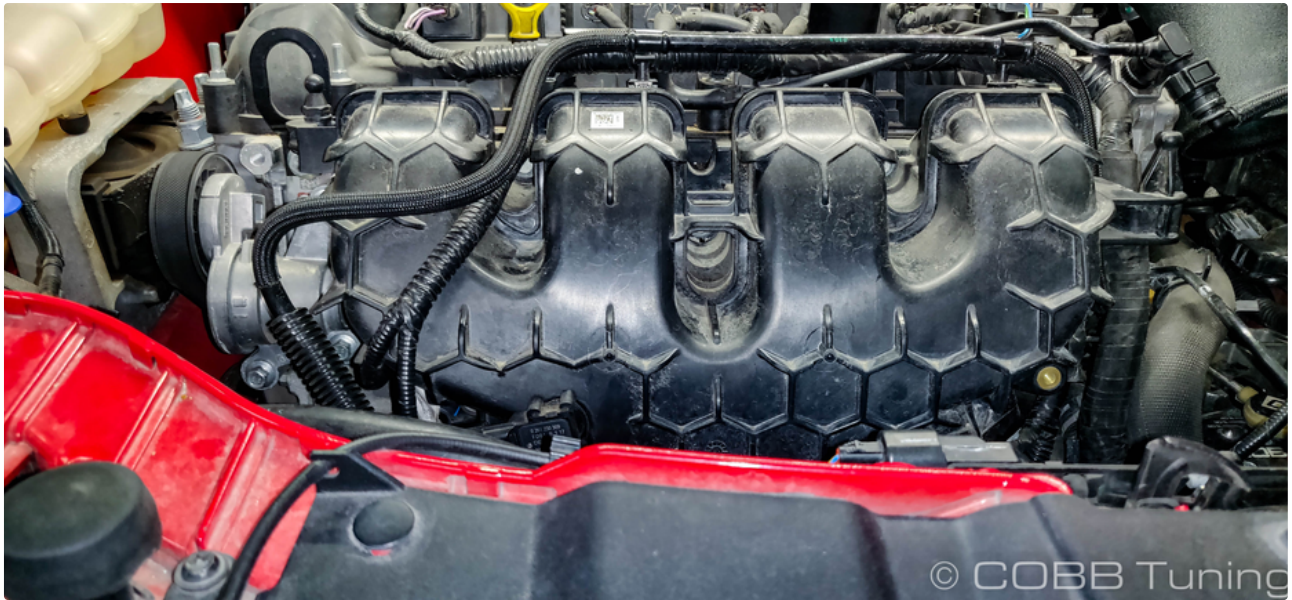
8. Remove the emissions line from the clips on top of the intake manifold.
