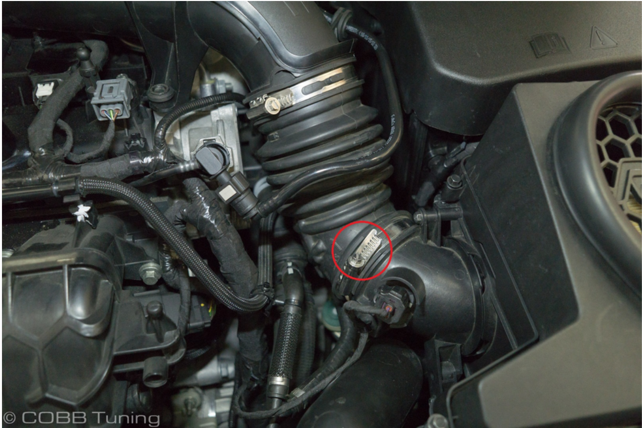
3. Loosen the hose clamp holding the intake pipe to the airbox. (7mm stock, 8mm COBB)
