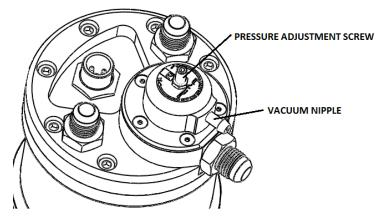
Re-install the FST pump fuse. Turn the ignition key ON. The lift pump and FST pump should prime at the same time. Check for leaks. Watch the pressure gauge during this time. Make adjustments to the pressure adjustment screw using a 3/32" Allen wrench, until proper fuel pressure is obtained. Several priming cycles may be necessary to allow an adjustment and reach the desired pressure.
