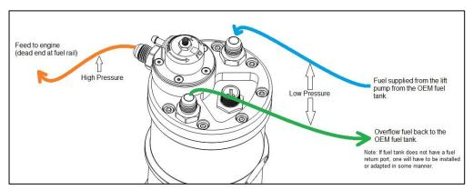
The FST-R has three -6AN ORB ports, these ports come by default with 6AN male adapters installed. Other adapters can be used as well but must be purchased separately. To complete the installation, -6AN (3/8") hoses will need to be constructed. The two -6AN ports on top of the fuel surge tank (shown in blue and green) are interchangeable. One port receives fuel from the main tank's "lift" pump and the other port is for fuel returning back to the main fuel tank. The side port on the FST-R
