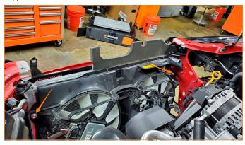
**04.** Refill and bleed the cooling system. The installation is now complete.
