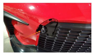
**05.** Using a 16mm socket, attach the license plate bracket to the rod with the supplied M10 hex head bolt & washer.
