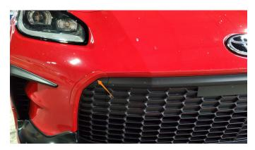
02. Remove the lower section of the tow hook cover.
