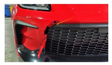
**03.** Remove both sections of the tow hook cover from the vehicle by releasing the tabs attaching the covers to the bumper.
