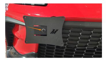
**06.** Using a 4mm hex key, attach your license plate to the license plate bracket with the four (4) supplied M6 button head flanged bolts.
