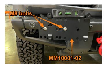
4. Fasten the front license plate to MM10001-02 with the provided M6 bolts.
