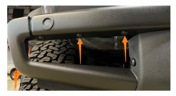
2. Fasten MM10002-01 to the bumper in the desired orientation using the T40 Torx bolts previously removed in step 1.
