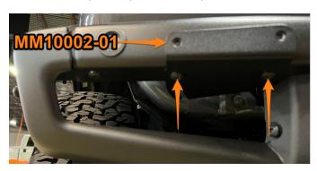
3. Fasten MM10001-02 to MM10002-01 in the desired orientation using the provided M8 bolts. A level should be used to ensure a nice, clean installation.
