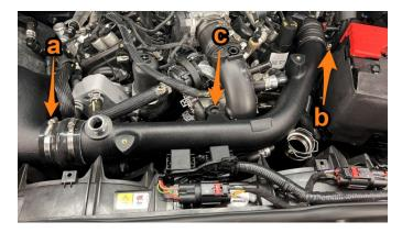
**15.** Using a 7mm socket, loosen the clamp on the passenger-side turbo.
