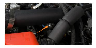
**34.** Install the lower boot of the assembly from step 32 onto the hotside pipe coming from the intercooler, then slide the upper right boot onto the pipe from the previous step.
