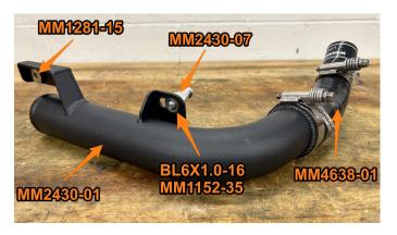
30. Install boot 2 onto hot-side pipe 2 then slide a 79mm clamp and 54mm clamp over the boot. Using a 3mm Allen wrench, install the 3 grub screws into the housing until they bottom out. Install the two grommets into the brackets.
