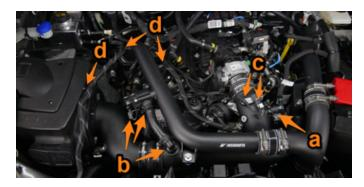
**40.** Loop one zip tie around the Mishimoto intercooler pipe on the driver-side. Loop another zip tie through the first one and around the vacuum hose. Pull tight and trim the ends. Repeat this process for the other vacuum hose.
