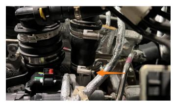
12. Remove the vacuum hoses from the two clips (a). Lift up and rotate the driver-side intercooler pipe back and forth to free it from the rubber mount (b). Remove the pipe from the vehicle.
