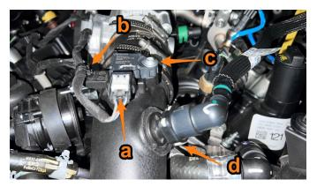
**14.** Using a 7mm socket, loosen hose clamps (a) and (b). Using an 8mm socket, remove bolt (c). Remove the intake pipe.
