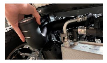
**25.** Once in position, slide the boots onto the intercooler adapters. The pipes should be inserted such that the edge of the boot is lined up with the 1 st white line from the end of the pipe. Tighten the clamps.
