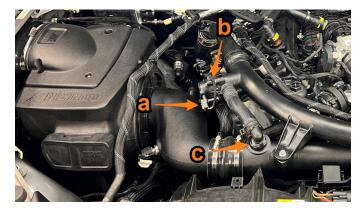
10. Using an 8mm socket, remove the three bolts securing the hot-side intercooler pipe to the air intake (a). Using a 7mm socket, loosen the hose clamp (b). Release the quick disconnect clip (c) and lift the passenger-side hot-side intercooler piping assembly out of the vehicle. (Image on top right)
