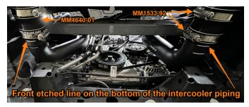
26. Using a 10mm socket and wrench, fasten the passenger-side intercooler pipe to the bracket with the provided 6mm bolt and nut. Install the longer straight section of boot 5 onto the pipe and slide 2x 92mm clamps over the boot.
