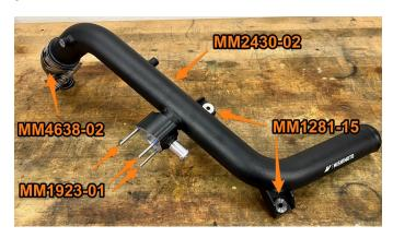
**31.** Using a 10mm socket, install the stock recirculation valve into the housing with the provided locking nuts.
