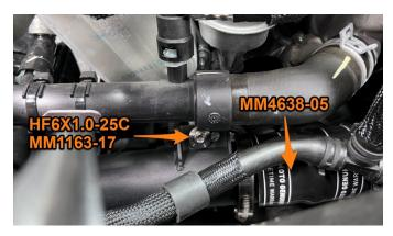
27. Install boot 6 onto the throttle body and slide 2x 92mm clamps over the boot. Insert the bottom of cold-side pipe 2 into the boot from the previous step then rotate the top into the boot on the throttle body. After ensuring proper alignment, use a 10mm socket to tighten all the clamps on the cold-side pipes. Using a 10mm socket, install the stock sensor into port (a) using the provided 6mm bolt, HF6X1.0-20A.
