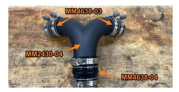
**33.** Install the assembly from step 29 on the driver-side of the engine, being sure to get the peg into the rubber grommet on the intake pipe and the boot onto the turbo outlet. The peg can slide in its slot to accommodate proper alignment.
