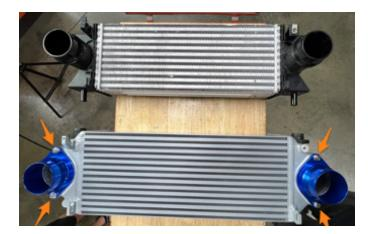
**6.** Remove the fan shroud from the stock intercooler and install it onto the Mishimoto intercooler using the provided hardware. (1x HF6X1.0-20A, 1x B4X0.7-16B)
