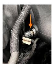
17. Using a 7mm socket, loosen the hose clamp on the throttle body (left image below). Using an 8mm socket on the bolt and 10mm wrench from behind the bracket to hold the nut in place, remove the bolt (right image below) Use a 7mm socket to loosen the hose clamp (right image below). Remove the upper cold-side intercooler pipe section.
