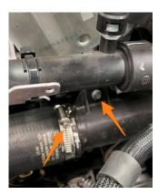
**18.** Using an 8mm socket, remove the bolt holding the ground strap and tuck the strap on top of the cross member.
