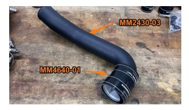
**24.** From the bottom of the vehicle, install cold-side pipe 1 on the passenger side and hot-side pipe 3 on the driver side. Reattach the ground strap from step 18.
