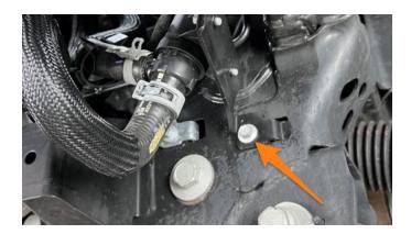
**22.** Install a grommet onto cold-side pipe 1 as shown by first installing the rubber part then inserting the metal sleeve.
