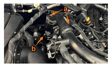
9. Unplug the recirculation valve connector (a) and remove the two wire clips (b). Disconnect the recirculation hose quick disconnect fitting from the air intake (c). Using an E5 Torx or 4mm socket, remove the 3 stud bolts and remove the valve from the stock intercooler pipe.
