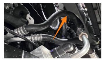
**21.** Using an 8mm socket, remove this bolt and tuck the hose/bracket out of the way.
