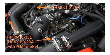
**38.** Using a 10mm socket, tighten all the hot-side pipe clamps. The clamp on the driver-side turbo outlet can be accessed through a hole in the fender liner.
