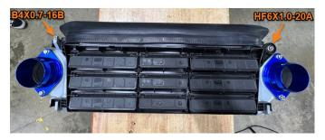
**06.** Remove the fan shroud from the stock intercooler and install it onto the Mishimoto intercooler using the provided hardware. (1x HF6X1.0-20A, 1x B4X0.7-16B)
