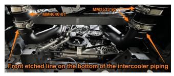
21. Using a 10mm socket and wrench, fasten the passenger-side Intercooler pipe to the bracket with the provided 6mm bolt and nut. Install the longer straight section of boot 5 onto the pipe and slide 2x 92mm clamps over the boot.
