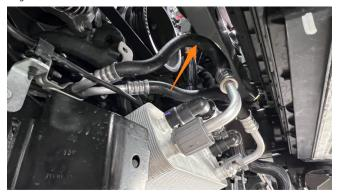
**14.** Using an 8mm socket, remove this bolt and tuck the hose/bracket out of the way.
