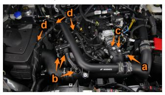
**35.** Loop one zip tie around the Mishimoto Intercooler pipe on the driver-side. Loop another zip tie through the first one and around the vacuum hose. Pull tight and trim the ends. Repeat this process for the other vacuum hose.
