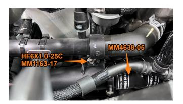
22. Install boot 6 onto the throttle body and slide 2x 92mm clamps over the boot. Insert the bottom of cold-side pipe 2 into the boot from the previous step then rotate the top into the boot on the throttle body. After ensuring proper alignment, use a 10mm socket to tighten all the clamps on the cold-side pipes. Using a 10mm socket, install the stock sensor into port (a) using the provided 6mm bolt, HF6X1.0-20A.
