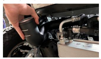
**20.** Once in position, slide the boots onto the Intercooler adapters. The pipes should be inserted such that the edge of the boot is lined up with the 1st white line from the end of the pipe. Tighten the clamps.
