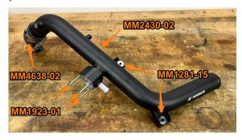
**26.** Using a 10mm socket, install the stock recirculation valve into the housing with the provided locking nuts.
