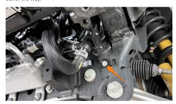
**15.** Disengage the quick disconnect fittings on the lower charge pipes and remove the pipes by pulling out from the bottom of the vehicle.
