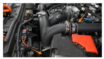
**30.** Install the assembly from steps 25/26 on the passenger-side of the engine, being sure to get the boot onto the turbo outlet and the other end of the pipe into the other side of the "Y" from the previous step.
