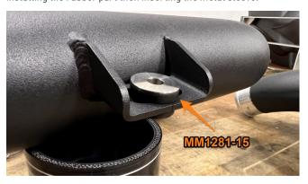
**17.** Swap the quick disconnect adapters on the Mishimoto stock-location Intercooler for the silicone boot adapters. Torque the bolts securing the adapters to the Intercooler to 10Nm (88.5 in-lbs).
