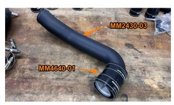
**19.** From the bottom of the vehicle, install cold-side pipe 1 on the passenger side and hot-side pipe 3 on the driver side. Reattach the ground strap from step 11.
