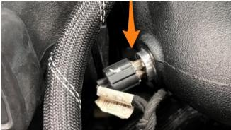
10. Using a 7mm socket, loosen the hose clamp on the throttle body (left image below). Using an 8mm socket on the bolt and 10mm wrench from behind the bracket to hold the nut in place, remove the bolt (right image below) Use a 7mm socket to loosen the hose clamp (right image below). Remove the upper cold-side Intercooler pipe section.
