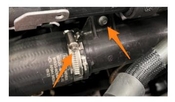
**11.** Using an 8mm socket, remove the bolt holding the ground strap and tuck the strap on top of the cross member.
