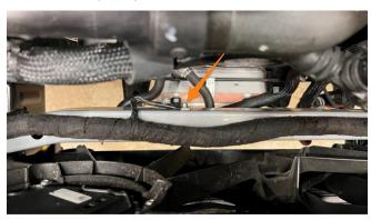
**12.** Using a 15mm socket, loosen the 2 rear bolts and completely remove the rest of the bolts. Remove the front skid plate/splash guard. Both the plastic splash guard and metal skid plate are shown below.
