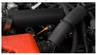
**29.** Install the lower boot of the assembly from step 27 onto the hot-side pipe coming from the Intercooler, then slide the upper right boot onto the pipe from the previous step.
