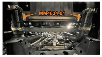
**20.** Using a 10mm socket and wrench, fasten the passenger-side intercooler pipe to the bracket with the provided 6mm bolt and nut. Install the longer straight section of boot 5 onto the pipe and slide 2x 92mm clamps over the boot.
