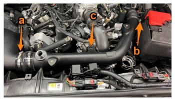
**8.** Using a 7mm socket, loosen the clamp on the passenger-side turbo.
