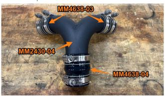
**27.** Install the assembly from step 23 on the driver-side of the engine, being sure to get the peg into the rubber grommet on the intake pipe and the boot onto the turbo outlet. The peg can slide in its slot to accommodate proper alignment.
