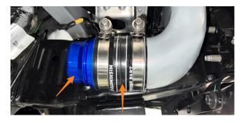
**18.** From the bottom of the vehicle, install cold-side pipe 1 on the passenger side and hot-side pipe 3 on the driver side. Reattach the ground strap from step 11.
