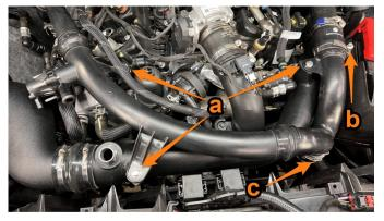
**4.** Through the driver-side wheel well, use a 7mm socket to loosen the hose clamp.
