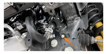
**15.** Disengage the quick disconnect fittings on the lower charge pipes and remove the pipes by pulling out from the bottom of the vehicle.
