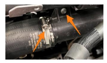
**11.** Using an 8mm socket, remove the bolt holding the ground strap and tuck the strap on top of the cross member.
