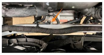
**12.** Using a 15mm socket, loosen the 2 rear bolts and completely remove the rest of the bolts. Remove the front skid plate/splash guard. Both the plastic splash guard and metal skid plate are shown below.
