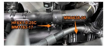
21. Install boot 6 onto the throttle body and slide 2x 92mm clamps over the boot. Insert the bottom of cold-side pipe 2 into the boot from the previous step then rotate the top into the boot on the throttle body. After ensuring proper alignment, use a 10mm socket to tighten all the clamps on the cold-side pipes. Using a 10mm socket, install the stock sensor into port (a) using the provided 6mm bolt, HF6X1.0-20A.
