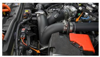
**29.** Install the assembly from steps 24/25 on the passenger-side of the engine, being sure to get the boot onto the turbo outlet and the other end of the pipe into the other side of the "Y" from the previous step.
