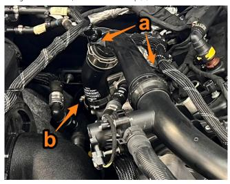
2. Unplug the recirculation valve connector (a) and remove the two wire clips (b). Disconnect the recirculation hose quick disconnect fitting from the air intake (c). Using an E5 Torx or 4mm socket, remove the 3 stud bolts and remove the valve from the stock intercooler pipe.
