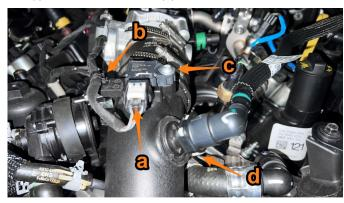
7. Using a 7mm socket, loosen hose clamps (a) and (b). Using an 8mm socket, remove bolt (c). Remove the intake pipe.
