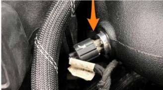
10. Using a 7mm socket, loosen the hose clamp on the throttle body (left image below). Using an 8mm socket on the bolt and 10mm wrench from behind the bracket to hold the nut in place, remove the bolt (image below) Use a 7mm socket to loosen the hose clamp (top image in next coloumn). Remove the upper cold-side intercooler pipe section.
