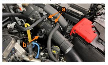
**6.** Unplug connector (a) and use a trim clip tool to remove tree clip (b). Using a T25 Torx, remove screw (c) and remove the sensor from the upper cold-side intercooler pipe.
