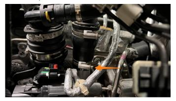
**5.** Remove the vacuum hoses from the two clips (a). Lift up and rotate the driver-side intercooler pipe back and forth to free it from the rubber mount (b). Remove the pipe from the vehicle.
