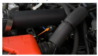
**28.** Install the lower boot of the assembly from step 26 onto the hotside pipe coming from the intercooler, then slide the upper right boot onto the pipe from the previous step.
