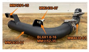
**24.** Install boot 2 onto hot-side pipe 2 then slide a 79mm clamp and 54mm clamp over the boot. Using a 3mm Allen wrench, install the 3 grub screws into the housing until they bottom out. Install the two grommets into the brackets.
