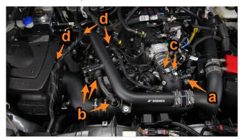
**34.** Loop one zip tie around the Mishimoto intercooler pipe on the driver-side. Loop another zip tie through the first one and around the vacuum hose. Pull tight and trim the ends. Repeat this process for the other vacuum hose.
