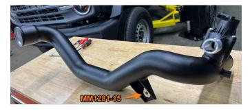
**15.** Using the provided clamps and turbo boot, install the Mishimoto hot-side intercooler pipe. Do not tighten the clamps, this will be done later. Reconnect the bypass valve hose and electrical harness.
