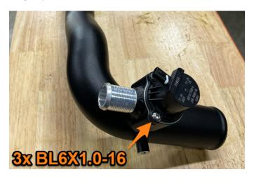
**14.** Install the provided grommet to the Mishimoto hot-side intercooler pipe. (MM1281-15)
