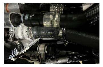
15. Install the driver side intake tube and silicone coupler. Use the original bolt for the bracket with pre-installed rubber grommet.Reconnect the surge valve fitting. (Second image on top right)
