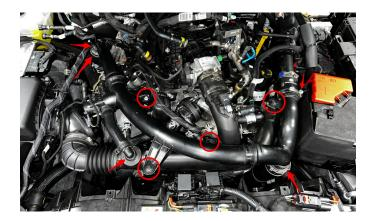
**10.** Loosen the worm gear clamp, then remove the driver-side intake hose. **(Second image on top right)**
