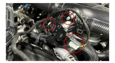
**07.** Lift the airbox straight up to disengage the rubber grommets at the bottom, and remove the airbox from the engine bay.
