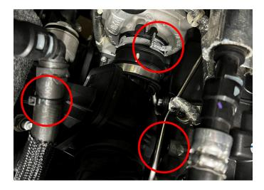
**09.** Remove the charge pipe. Release the tree clip holding the coolant hose to the charge pipe. Loosen the worm gear clamp near the battery. Disconnect the surge valve hose from the driver-side intake hose. Remove 4x 8mm bolts, then release the 2x spring clips to remove the charge pipe from the engine bay.
