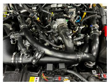
**17.** Tighten all 5x worm gear clamps on the Mishimoto intake, don't forget the one on the stock rubber coupler next to the battery.
