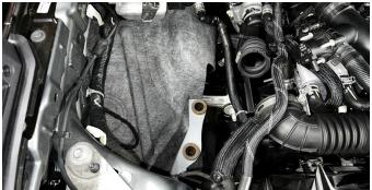
**08.** Remove the passenger side intake hose. Unclip the coolant hose, then remove the bolt securing the intake hose to the engine block. Use a spring clamp tool or pliers to open the spring clamp, then pull the hose from the turbo inlet. **(Second image on next page)**
