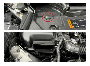
**02.** Remove 1x bolt holding the airbox to the fender frame.
