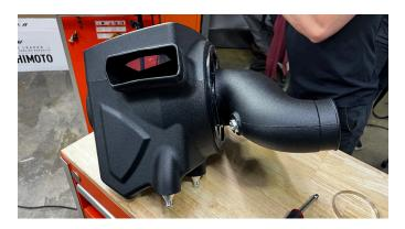
**12.** Install the Mishimoto airbox and split tube assembly to the stock location and push down on the airbox to engage the bottom pegs. Clip the coolant line tree clip to the side of the airbox as shown.
