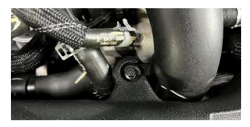
16. Reverse step 9 to reinstall the charge pipe. Use the 3x provided10mm hex head bolts to fasten the charge pipe to the Mishimoto intake pipe. Use the longer bolt on the grommet.
