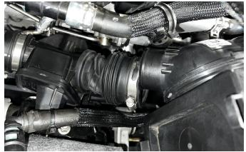
**06.** Unplug the surge valve harness and slide the retainers out from the studs. Move this harness out of the way to remove the airbox.
