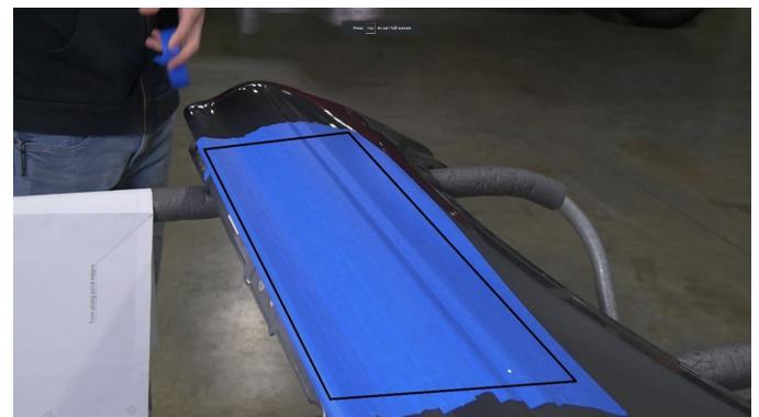
**42.** Coat the unprinted side of the template with a mild adhesive, like the 3M Super 77 spray adhesive or glue stick. Align the marked corner and front side of the template (a) with the mark made in the previous step (b).
