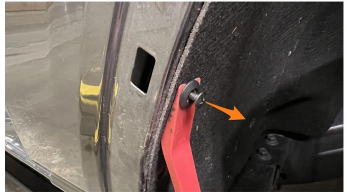
**18.** There are 3 screws located on the fender liner that needs to be removed.
