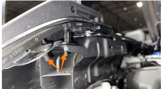
25. Using a 10mm socket, remove the 3 screws.
