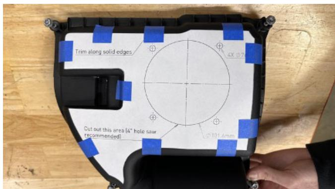
**33.** Using a center punch, mark the center of the large circle and the 4 small surrounding holes.
