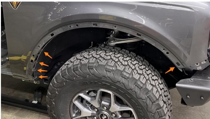
**16.** To remove these clips, use a Phillips head screwdriver to turn the plastic screw about 1/4 inch out. Apply just enough force to keep the driver in the head of the screw while turning. If too much pressure is applied, the screw will not thread out.
