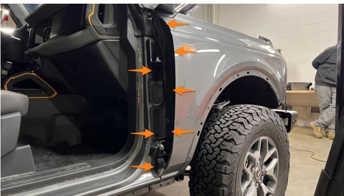
23. Using an 8mm socket, remove the upper screw, then use a 10mm socket to remove the 3 lower screws.
