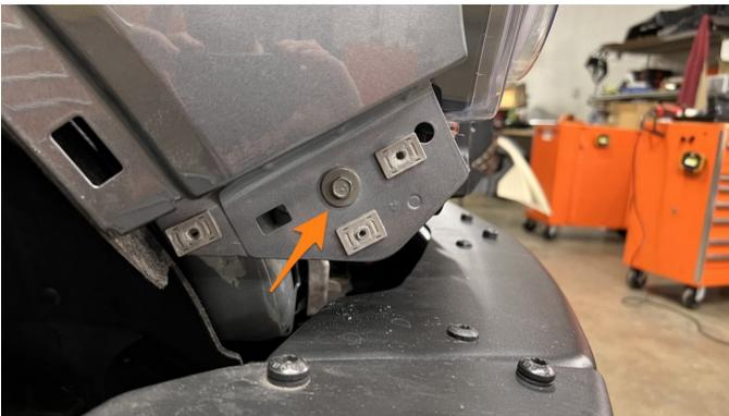
22. Using a 10mm socket and trim tool, remove the 3 screws and 4 clips. Next, pull out the cover panel.
