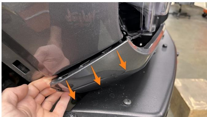
**10.** If equipped with rock sliders, the passenger side slider will need to be removed in order to access the bottom bolts for the fender. At the three locations shown below, use a 10mm socket to remove the two nuts (a) and a 13mm socket to remove bolt (b).
