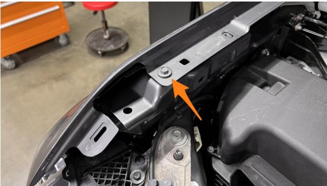
28. The fender can now be removed by pulling straight away from the vehicle. Be careful not to damage the small tab near the mirror while removing it.
