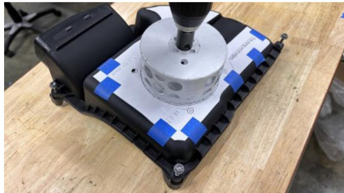
**36.** Once all the holes are drilled, remove the template. This is how the lid should look now.
