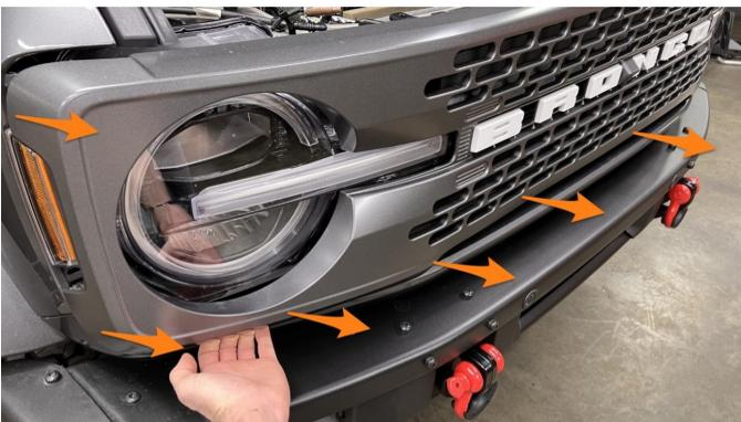
**07.** On the passenger side of the vehicle, rotate the 5 lock levers a ¼ turn toward the wheel. Once the levers are disengaged, remove the fender flare by popping the clips loose, starting at one end and working your way down to release the rest.
