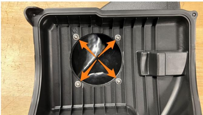
**39.** Using a 2.5mm Allen wrench, remove the 3 screws and clear lid from the Mishimoto intake.
