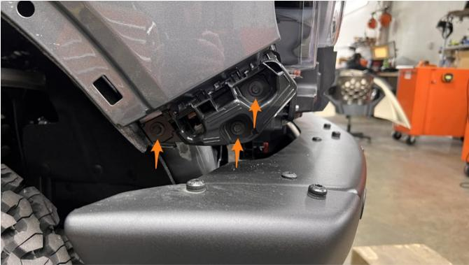
21. Using a 10mm socket, remove the screw that was behind the bracket.
