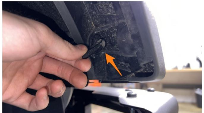
**08.** On the driver side, disengage the first two levers (toward the front) and pop the front of the fender flare loose.
