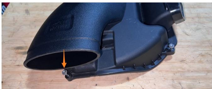
**53.** Reinstall the stock airbox assembly with the adapter inserted into the silicone coupler. Tighten the worm gear clamp. **If using a Mishimoto intake, skip to step 54. Skip to step 55.**
