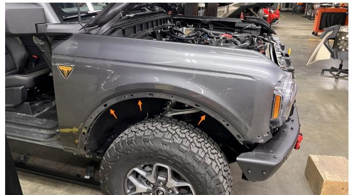
**19.** Using an 8mm socket, remove the 3 screws.
