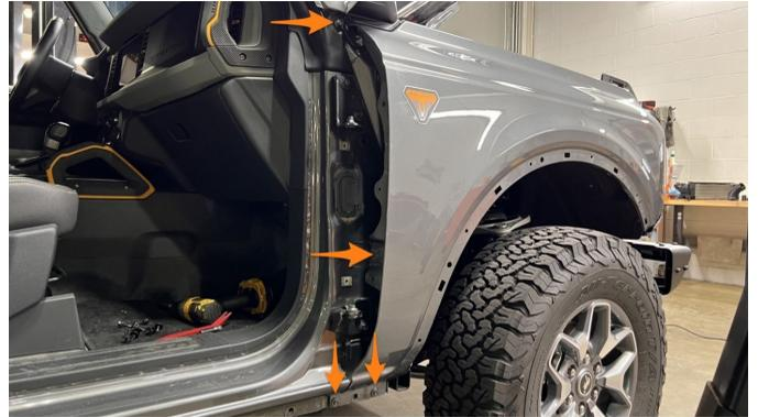
24. Using a 10mm socket, remove the 2 nuts.
