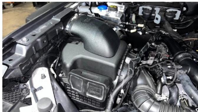
**54.** Install adapter 2 MM2437 into the coupler and onto the Mishimoto airbox. Using a 2.5mm wrench, fasten with the supplied M4 hardware (see parts diagram). Tighten clamp (a).
