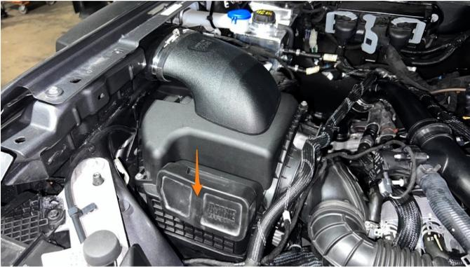
**56.** Install screen MM2383 onto snorkel head MM2379 with the supplied M4 hardware (see parts diagram). Slide t-bolt clamp MM1298-425 over the collar on the snorkel head.
