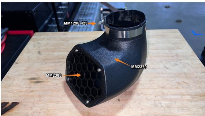
**57.** Install the snorkel head onto the snorkel and use a 10mm socket to tighten the clamp. Optionally, use the small rubber cap [MM1342-09] to cover the exposed stud on the clamp.
