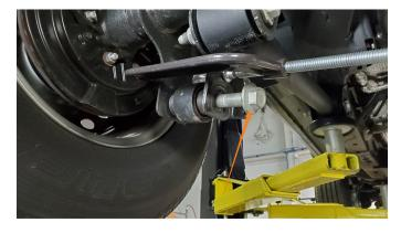
**03.** Install the skid plate onto the lower strut mount. The tab on the skid plate with the full hole will go onto the end of the strut mounting bolt as shown in the photo below. The "BORNE OFF-ROAD" logo faces the rear of the vehicle. (Image on next page)
