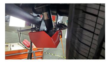
**04.** Install (2) supplied M10 bolts, (2) supplied flat washers, & (1) supplied bar nut as shown in the photo below. Tighten each bolt to 25 lb-ft (34 Nm).
