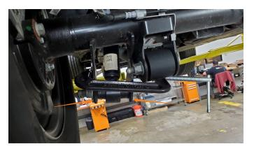
**02.** Using a 27mm socket loosen the driver side lower strut mounting bolt and remove the nut. A long breaker bar may be needed to get this bolt loose. The factory service manual recommends replacing this bolt and nut with a new bolt and nut when reinstalling.
