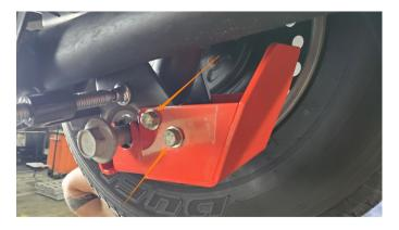
**05.** Loosely install the lower strut mount nut onto the end of the lower strut mount bolt then remove the clamp from the flanges. Do not fully tighten the lower strut mount bolt at this point.
