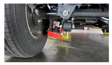
NOTE: If you do not have a torque wrench that reaches 350 lb-ft, tighten the bolt to 150 lb-ft and mark it as shown in the photo below. Then, tighten the bolt an additional half turn (180°).
