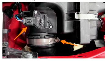
**3.** Using a 10mm socket, remove the air box mounting nut and two bolts. Disconnect the intake pipe and remove the airbox.
