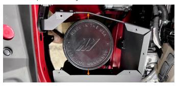
**19.** Once centered, use a 7mm socket to tighten the hose clamp for the intake pipe.
