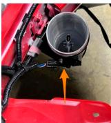
**17.** Using a 10mm socket. Install the airbox using the factory hardware and mount points.
