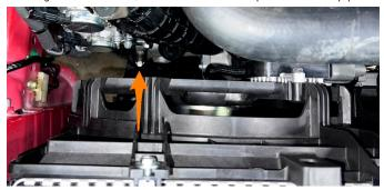
**6.** Using a 10mm socket, remove the nut for the intake pipe and pull the intake pipe out.
