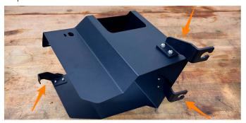
**12.** Install the rubber bushings from the stock airbox into the two bottom brackets.
