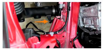
7. Using a T15 Torx, remove the two MAF sensor screws and remove the sensor from the airbox.
