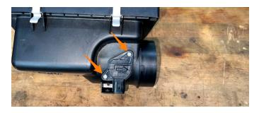
**8.** Undo the two airbox clips and separate the two halves. Using a 10mm socket, remove the rubber mount nut and mount.
