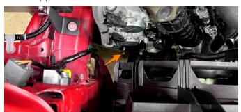
20. Using a 2.5mm Allen, install the airbox lid with the provided M4 hardware. Don't over-tighten. Install the factory airbox duct and pop clips.
