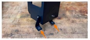
**13.** Using a 10mm socket, install the rubber mount from the stock airbox with the shouldered side in the slot.
