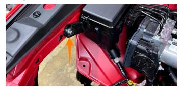
5. Using an 8mm socket, loosen the hose clamp on the intake pipe.
