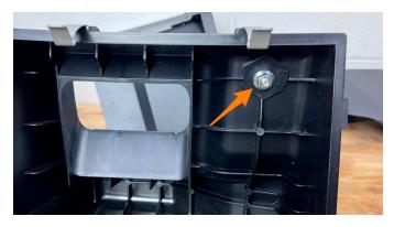
**9.** Remove the two rubber bushings from the airbox by first pushing the metal sleeve out.
