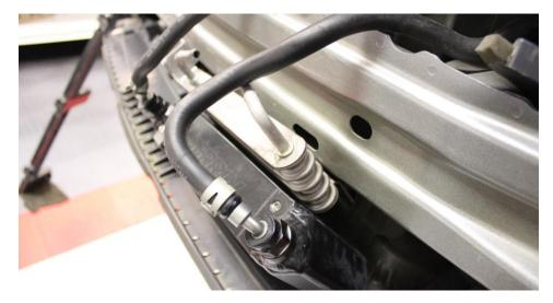
6. Locate upper radiator support and the (2) threaded holes where brackets will be mounted to. Drop oil cooler and hoses behind bumper beam and install oil cooler to core support using supplied M6 bolts and fender washers.
