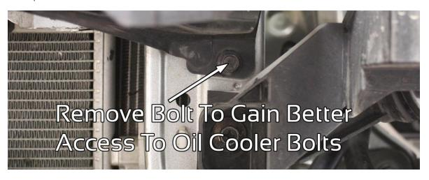
5. Locate and remove (3) M8 Bolts securing OEM oil cooler to chassis. NOTE: Depending on the tools that you have, you may want to remove the bolts securing the upper steel bumper support. See picture above showing bolts to remove on either side.
