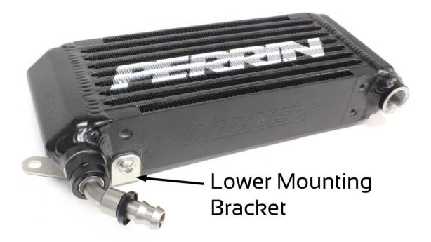
4. Install mounting brackets to PERRIN transmission cooler as shown. Secure brackets using supplied M8x10 bolts (not the longer M8x16 bolts as these will damage the core) and washers Take note of slots in brackets as some adjustments to the fitment may be necessary during the next few steps.
