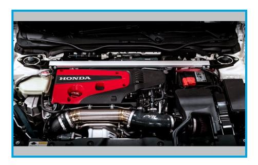
Depending on vehicle and chassis tolerances, fitment may be tight to the air ducting underneath the hood of the vehicle. Please inspect for clearance. If tight or contact is made, the thin tabs may need trimmed or simply bent out of the way ( can be pushed with fingers).
