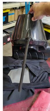
11. Slip clamps over both ends of the intake tube and then loosely slip it onto the airbox with the side with both fittings towards the airbox.
