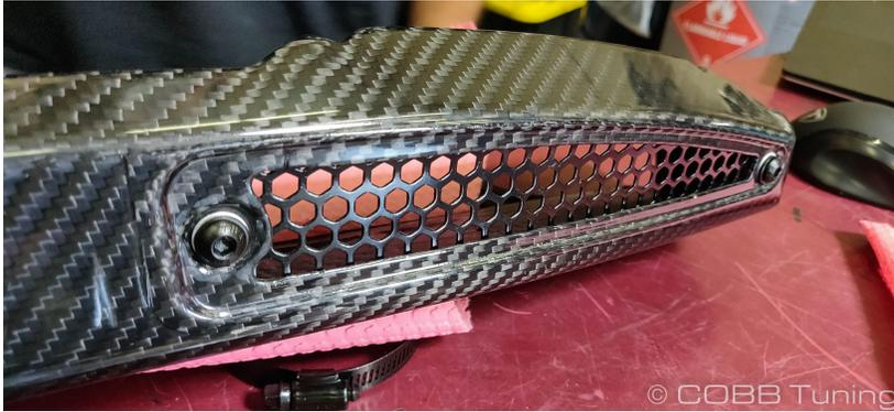
5. Use the provided foam tape to make a seal around the airbox lid. Make sure to stick to the provided flat area.
