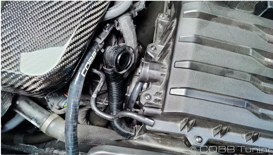
5. Unclip the air pump from the stock airbox.
