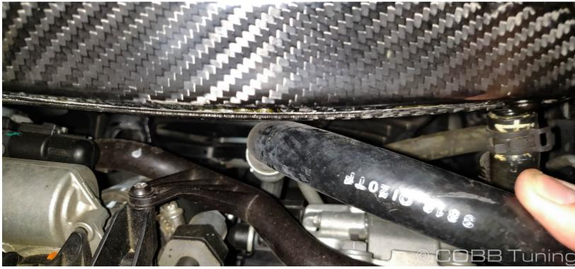
3. Connect the air pump (if equipped) to the bottom of the intake. You may need to carefully rotate the fitting in the tube, while doing so make sure to support the hose as you turn to avoid just twisting the tube itself.
