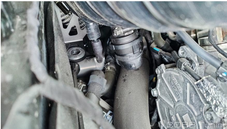
4. Connect the vacuum line from the intake silicon to the fitting where the factory vacuum line was connected.
