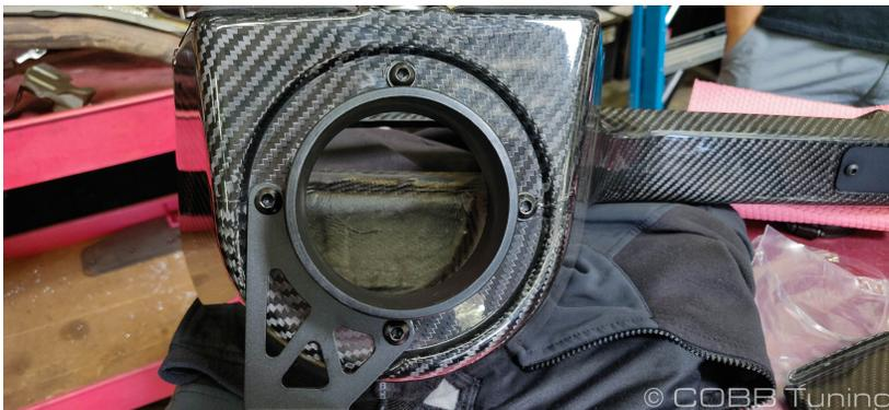
4. Looking at the back side of the airbox there is a removable panel. The factory panel allowed some air through this area to circulate in the engine bay so remove the two allen bolts if you'd like to keep this. If you're less worried about cooling the drivetrain you can close off this panel.
