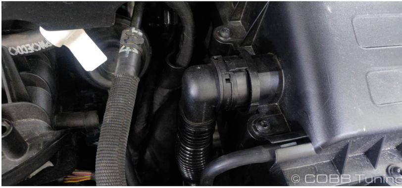
9. Add the provided small vacuum line to the small barbed fitting on the bottom of the intake silicone.
