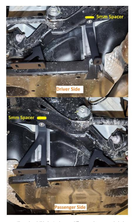
**2.5.** Next, we will need to drill holes in the rear diffuser so that we can bolt the suspension covers to it. Using 16mm long M6 BHCS, and serrated flange nuts, temporarily bolt one suspension cover to one set of brackets just installed (driver side or passenger side).
