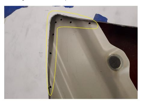
**2.10.** Following the Series of hole drilled in the previous steps, cut the "outline" that you have created in the previous step.
