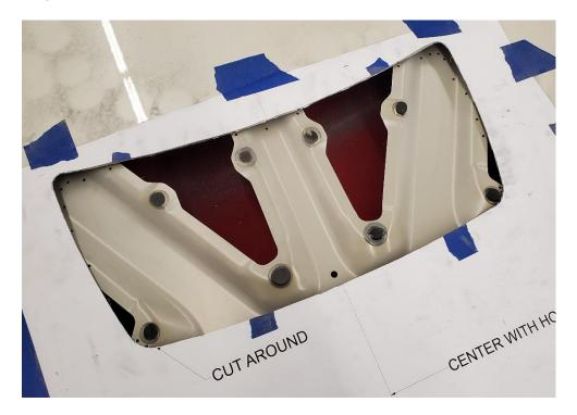
**2.8.** You may need to pull the cutout portion upward to release the bonded areas from the structure underneath.
