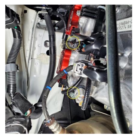
**2.8.** Unclip the O2 sensor harnesses from the brackets.
