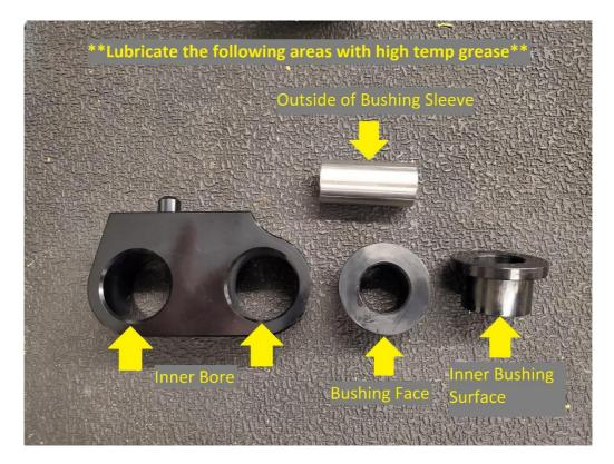
**2.4.4.** Insert the bushing halves (8) into the bushing retainers.
