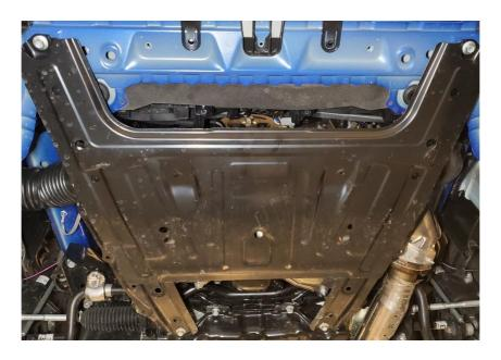
**2.9.** Begin by removing the front exhaust pipe.
