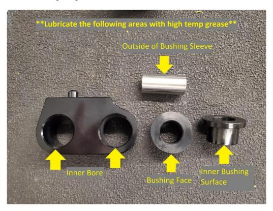
**2.4.4.** Insert the bushing halves (8) into the bushing retainers.
