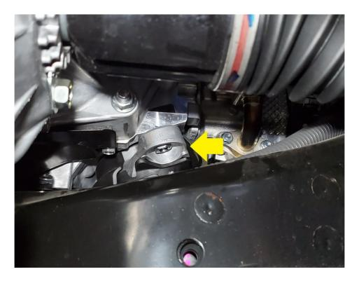
**2.16.** Install the Verus Engineering motor mount using the OEM 14mm head bolts. Torque to 26 ft-lbs. Make sure the locating dowels are facing the outside of the car.
