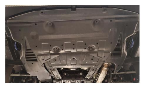
2.8. Remove the turbo cover plate. This is held on with 12mm bolts.
