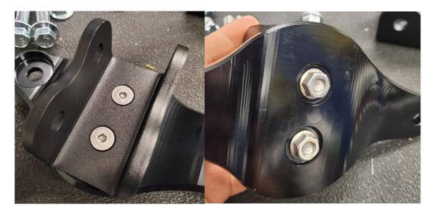
**2.4.2.** Three different durometer bushings are supplied. Which durometer you install is ultimately up to you, however we installed the black bushings. **Black – Soft, Grey – Medium, Blue – Hard**.
