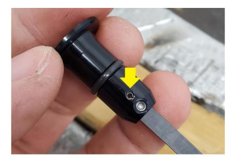
**2.6.** Next, to prevent the dipstick from wobbling around apply some Loctite to the supplied M3 set screw, and tighten it using a 1.5mm allen key. Just snugging up after bottoming the screw is sufficient. A dab of threadlocker is recommended.
