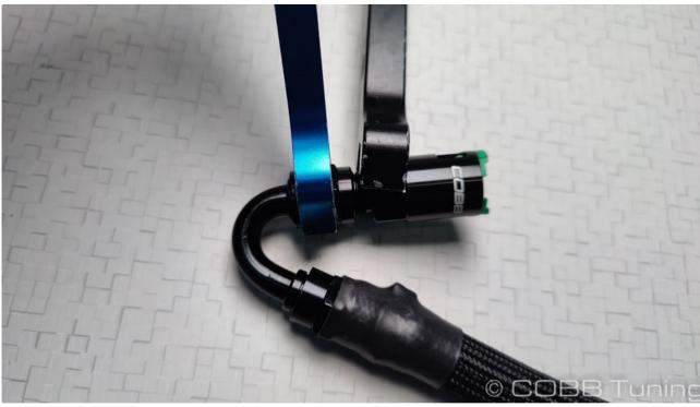
3. To remove the fitting from the ethanol content sensor in the future, all you'll need to do is squeeze the green part where it sticks out the back and pull the AN portion outwards. The green portion will stay on the ethanol sensor for reinstallation and the AN fitting will pop off. When re-seating the clip, make sure the tabs line up with the squared off holes. The tabs lining up is what retains the fitting when under pressure.
