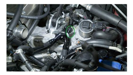
9. Some of your intake will need to be removed. If using a COBB SF intake, you can get by with just removing the silicon piece going from the maf housing, to the turbo inlet.
