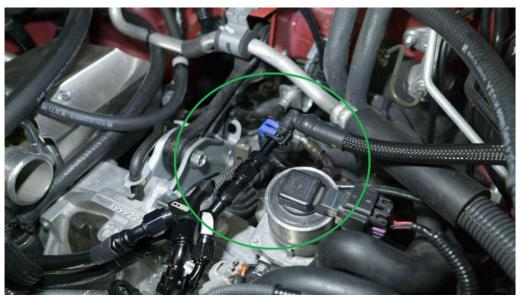
8. Using two -6 AN wrenches, remove the female to female adapter and quick connect fitting from the fuel rail lines. (This may need to wait until removal of the intercooler)
