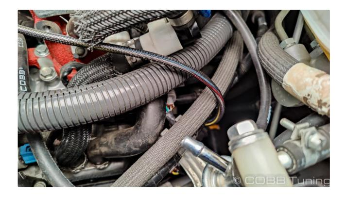
9. Pull the ethanol content sensor plug out underneath all the lines near where the battery tray was. It can get plugged into the ethanol content sensor.
