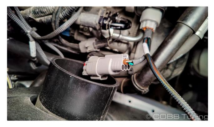
5. If you're using the fuel pressure sensor kit, plug the flex fuel harness into the fuel pressure sensor harness, then the fuel pressure harness into the engine harness. If these are not done in the correct order you will end up getting error codes pop up.
