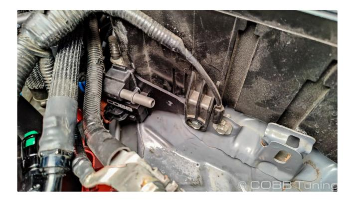
5. Now you can push the fuel line with the green connector installed onto the ethanol content sensor.
