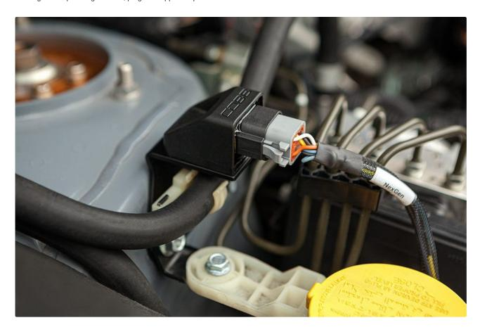
2. Working down the harness making sure not to route it too tightly between things as the engine will move. Unplug the factory connection from the TGV. There is a release to squeeze on the bottom side of the connector.
