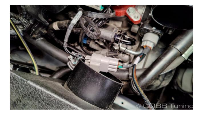
6. The next plugs as you head down the harness will go to the electronic boost control solenoid (EBCS). These plug into the harness and EBCS to provide power for the flex fuel system. It's possible to get this unplugged without undoing the bracket from the intake manifold, but it can be easier to see what you're doing if you do remove the bracket. To do so it's a 12mm near the coolant tank, and a 10mm on the front side.
