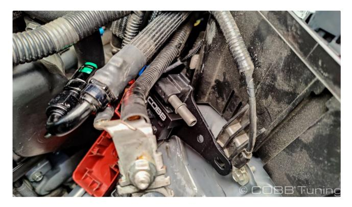
4. Now slip the ethanol content sensor with the blue fuel line and electrical connector attached, under the tab for the fuse box, and tighten it back down with the factory bolt.
