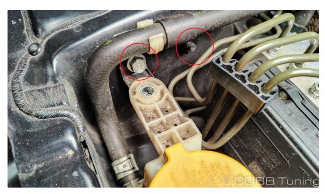
2. Slide the right hand side of the module bracket over the stud on the engine side, then rotate it downwards until it's behind the bolt on the outside.
