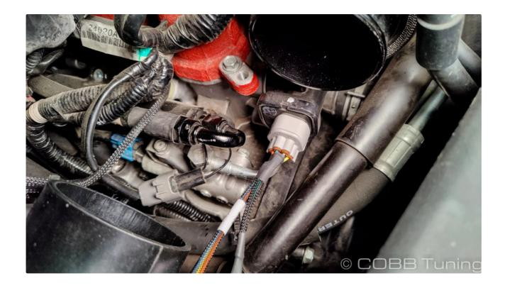
4. Now if you're running it without the fuel pressure sensor, plug the flex fuel harness into the stock engine harness.
