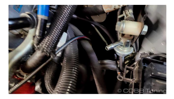
3. The blue end can get run down to the flex fuel sensor and the clip pushed shut. This should install to the same end as the electrical connector.
