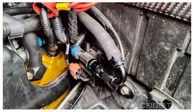
6. Make sure the fuel line stays relatively close to the fuse box, and route it through the other cables and hoses over to the back of the motor, where you can re-attach it to the AN y-fitting (or fuel pressure sensor adapter)
