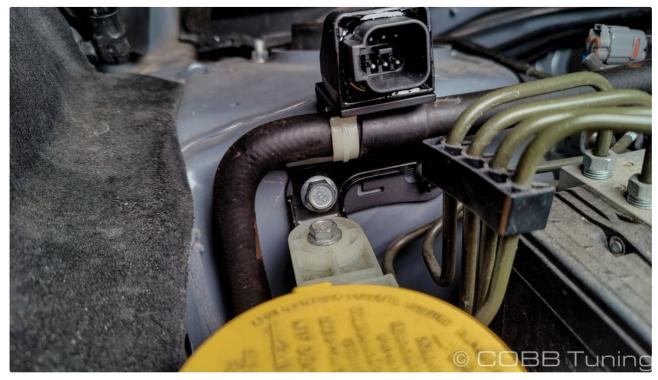
${\it 3. Once the module bracket is snug behind the stock bracket, you can snug the bolts back down.}\\$
