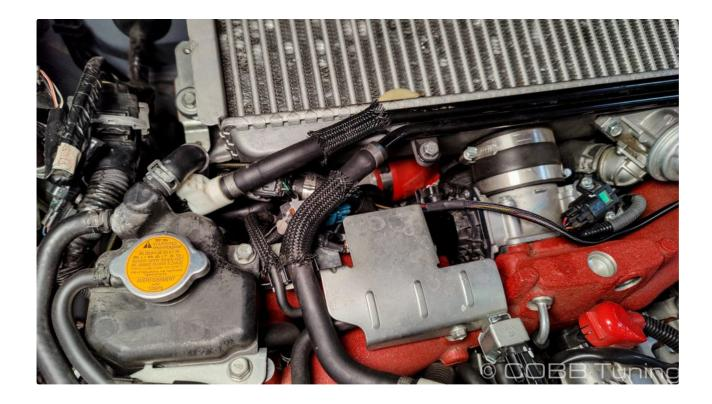
8. Once your wires have made it to the driver's side (USDM). Take a second (or several minutes for those of us with large hands) and remove the engine harness connector from the TGV. Once again, the harness will go in-between the engine harness and TGV. It's usually easier to connect to the TGV first, and then the engine harness. You'll also want to pull the brown ethanol sensor connector down there and the ground so you can route both under the battery cables and fuel lines to prevent chafing.
