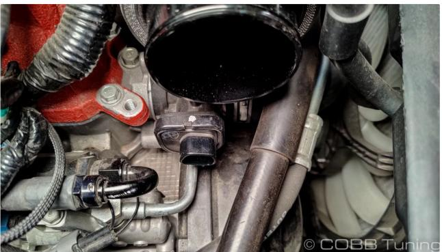
3. Plug the Flex Fuel harness into the TGV directly.
