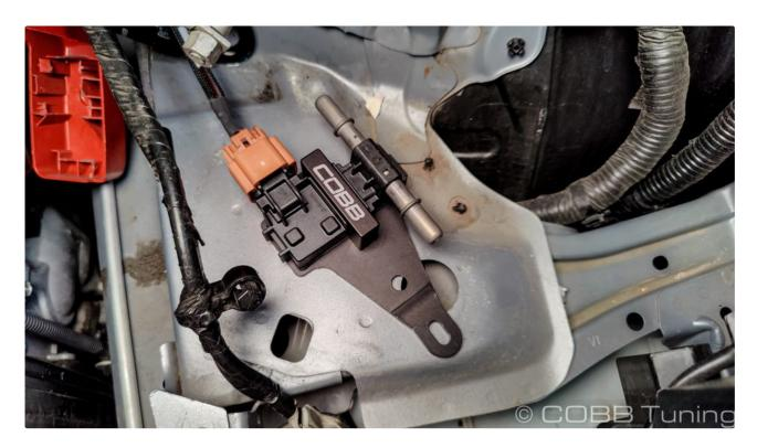
10. Run the small ground wire underneath everything and up the back side of the fuse box to sit under the 10mm bolt sitting next to the main fuse box bolt. (the cover will need to be off to remove that bolt)
