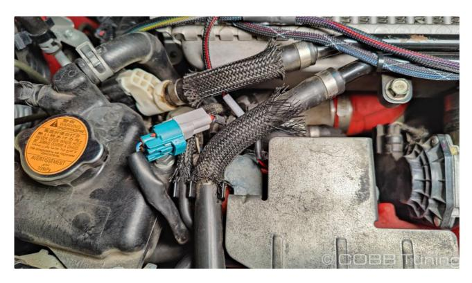
7. You can either run your wires along the pcv hoses on top of the intercooler (in which case you'll pull them out of the way for now, keep in mind you'll need to trim zip ties every time you remove the intercooler) OR along the top point of the intake manifold and meet up with the MAP sensor harness.
