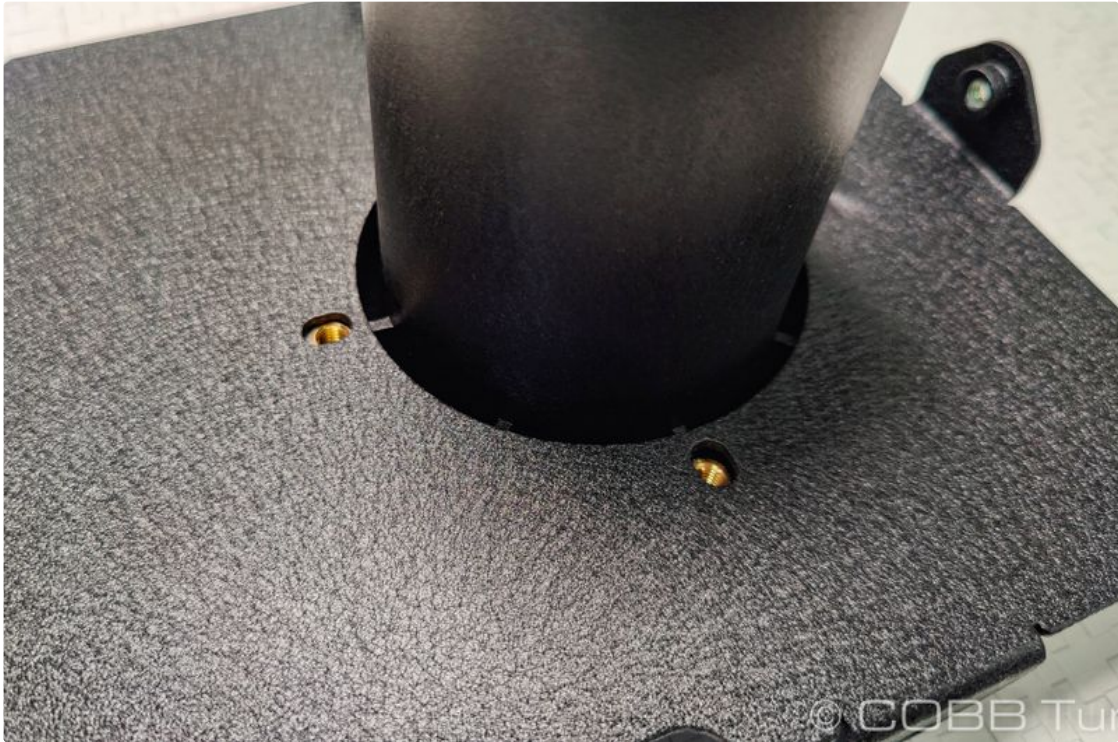
The back side with the longer end and the MAF opening should be on the same side that there are two flat tabs sticking up.
