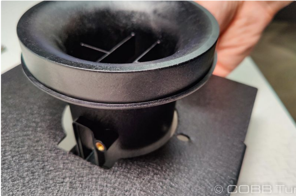
The back side with the longer end and the MAF opening should be on the same side that there are two flat tabs sticking up.
