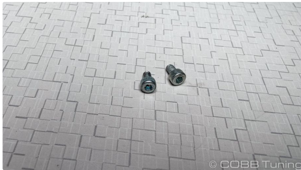
▼ (2) m4 x 6mm socket head MAF Bolts
