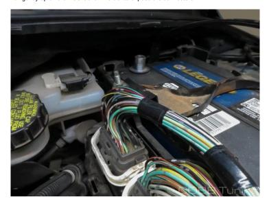
5. Push in on the lowest (barely exposed) tab on the electrical connector and pull up on the white arm to release the plug from the ECU.
