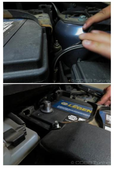
3. Remove the battery from the battery box.
