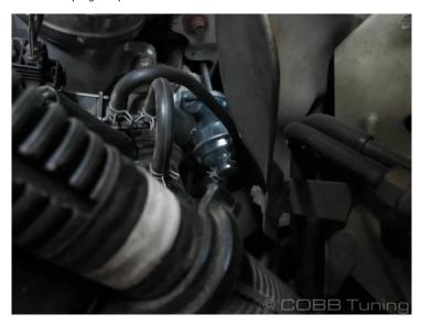
5. Carefully undo the hard to get to clamp on the inlet where it hooks up to the turbo. Then remove the inlet tube from the car.
