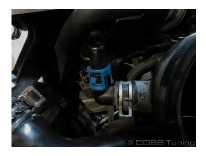
8. With the 10mm remove the clamp holding the intake to the turbo inlet and pull the intake tube free from the car.
