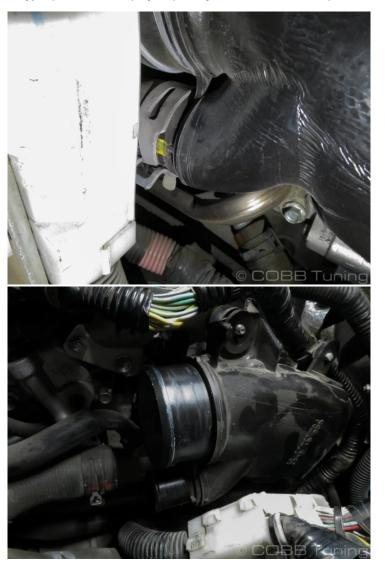
3. Remove the 10mm bolt holding the inlet to the engine.
