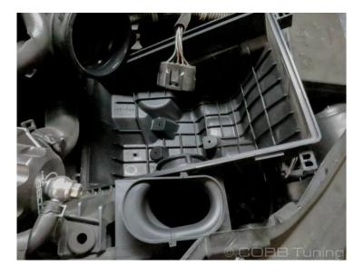
6. Pull firmly upwards on the lower airbox in order to pop it free form the rubber grommets it sits in.
