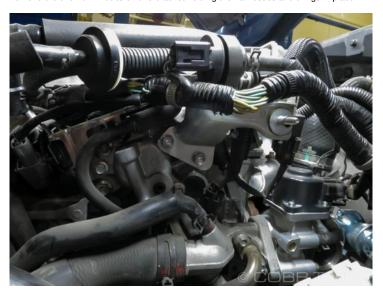
2. Disconnect the electrical connector from the top of the HPFP.
