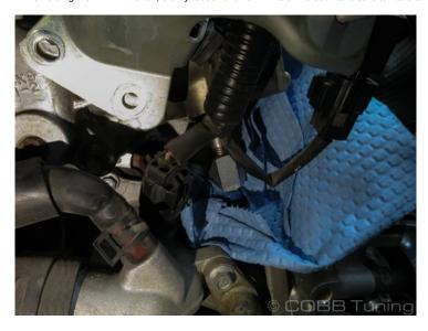
5. Undo the two fuel lines from the top of the HPFP by popping off the plastic retaining collar and pull the fuel line free.
