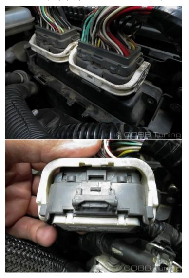
6. Using a pair of needlenose pliers gently squeeze the grey tabs and release the wiring harness from the battery box.
