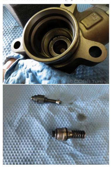
${\bf 4.} \ {\bf Starting} \ {\bf at} \ {\bf the} \ {\bf back} \ {\bf end}, \ {\bf you} \ {\bf can} \ {\bf remove} \ {\bf the} \ {\bf black} \ {\bf pump} \ {\bf spacer} \ {\bf from} \ {\bf the} \ {\bf pump} \ {\bf itself}.$
