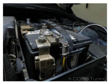
2. Still using the 10mm remove the battery bracket.
