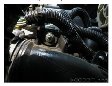
4. Remove the spring clamp and electronic boost control solenoid line.
