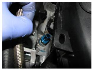
**2.9.** Remove the other side of the PCV system, which goes from the block (via a black plastic fitting under the A/C compressor) to the intake tube. It is the hose drawn in yellow and circled in yellow below. **It may be easier to remove the AC compressor, remove the belt and unbolt the compressor. We used <b>45 degree needle nose pliers.**
