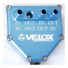
Note: If at any point you get confused about how the hoses should be routed into the AOS unit, just remember that the AOS acts as an inline filter. This means that the pathway for air should always flow from the engine > into the AOS > back into the engine. For example, on the PCV side, crankcase air will flow out of the engine block, into and through the AOS, out of the PCV valve (installed in the AOS), and back into the intake manifold.
