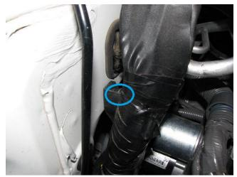
**2.11.** Using the supplied M6x1.0 BHCS and 18mm washer on the bottom point, slide the top/side bracket behind the point mentioned above. You will have to install the stock bracket removed in step **2.5**. Securely tighten these two points when the bracket is nicely installed.
