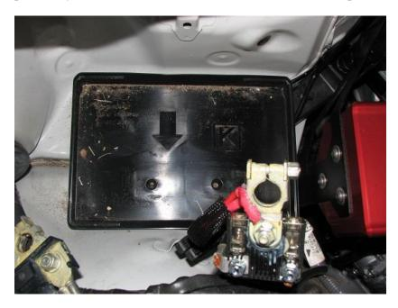
**2.5.** With the battery tray removed, you will want to fully remove the bracket shown below. Remove the two 10mm bolts circled in blue and then remove this bracket completely. We will re-use this bracket, do not throw it away.
