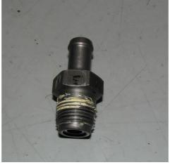
**2.8.** Install the supplied 3/8NPT to 1/2" adapter fitting. You will need a 7/8" deep socket to install this. It is recommended to use some Teflon tape or sealant to ensure a leak free seal as shown below. Install this adapter to 12-18 ft-lbs.
