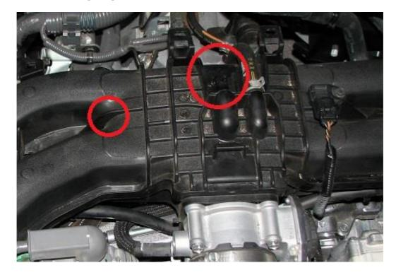
**2.7.** Remove the PCV valve using the 22mm deep socket, extension, wobble socket, and ratchet.
