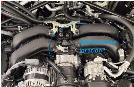
**4.6.** This will expose two barbs (one on the throttle body, and one on the coolant pipe) that we can use for the coolant circuit.
