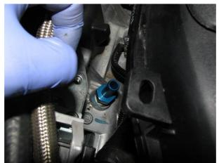
**2.9.** Remove the other side of the PCV system, which goes from the block (via a black plastic fitting under the A/C compressor) to the intake tube. It is the hose drawn in yellow and circled in yellow below.
