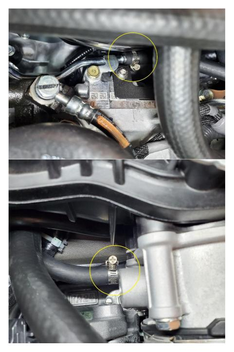
**4.7.** Cut two lengths of hose approximately 21" long, and 26" long. Refer to the diagram below for hose routing. Be sure to slide the clamps onto the hose before installing them.
