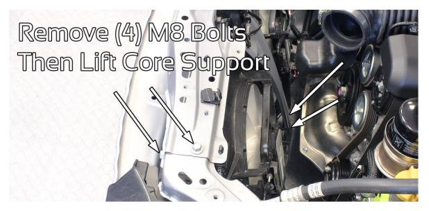
10. Lift up on left side of radiator support (leaving plastic intake air diverter in place) and place PERRIN intake tube under support as shown below. Make sure the tab on PERRIN intake is in front of radiator support and closely lines up to threaded M6 hole shown below. Carefully set radiator support back down and reinstall and tighten (4) 12mm bolts removed earlier.
