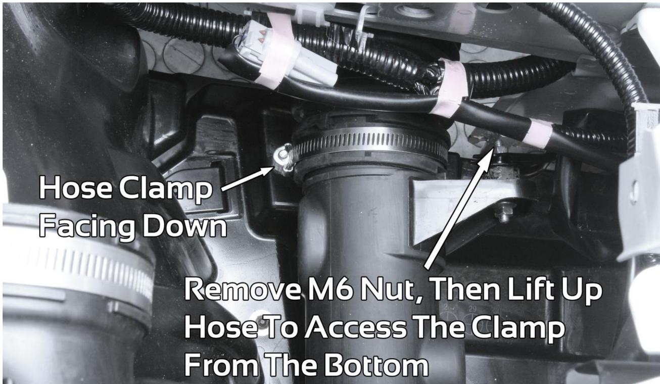
9. Remove OEM intake tube from chassis.
