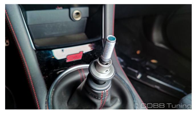
5. Thread the COBB Knob on clock-wise. until it stops. There is no need to overtighten as you can just rotate the ring until the logo is where you want it.
