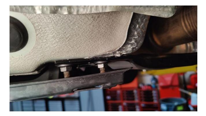
5. Undo the front exhaust joint. I'd recommend loosening the nuts until the clamp is free and breaking it loose from the pipes, but leaving it loose enough that it will support the front of the exhaust.
