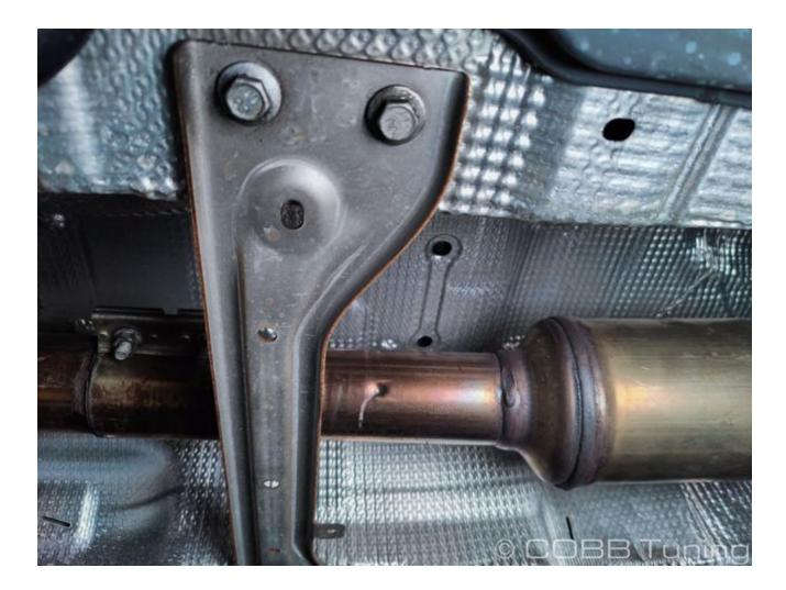
4. Near the rear of the car remove the rear cross brace as well. On some cars you'll need to sneak under it with a wrench or remove the undertray if you don't want to bend the plastic.
