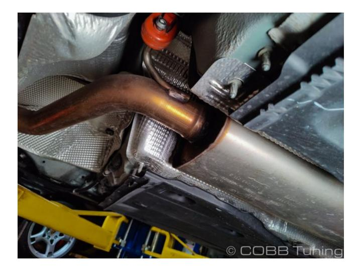
7. With a friend, jack, or both supporting the exhaust, use your 13mm and an extension to remove the exhaust hangers on either side of the muffler then drop the exhaust out of the car.
