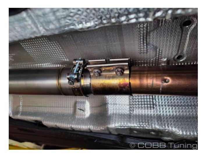
5. Add the muffler section into place popping it into the exhausting front exhaust hanger and the new urethane exhaust hanger.
