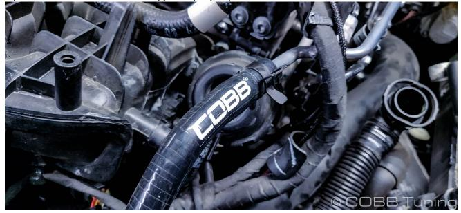
6. Once that's done you can move to the end where you removed the clamp earlier. Gently spin the line to break it free from the radiator hose, be careful as the connection is plastic and may be brittle if the vehicle is older. Once done you can pull off that end of the line and do your best to minimize spills while quickly installing the new line onto the radiator hose. Any Indiana jones references you make while doing so earn double points.
