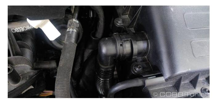
7. Now you should be able to pull the stock airbox and intake tube out of the car by popping the box off of the grommets that hold it in place.
