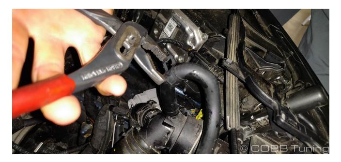
7. You should now be free to install the other end and secure with the provided spring clamp.
