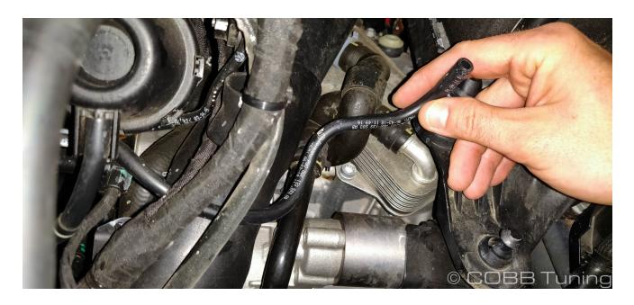
6. Unclip the air pump from the stock airbox.
