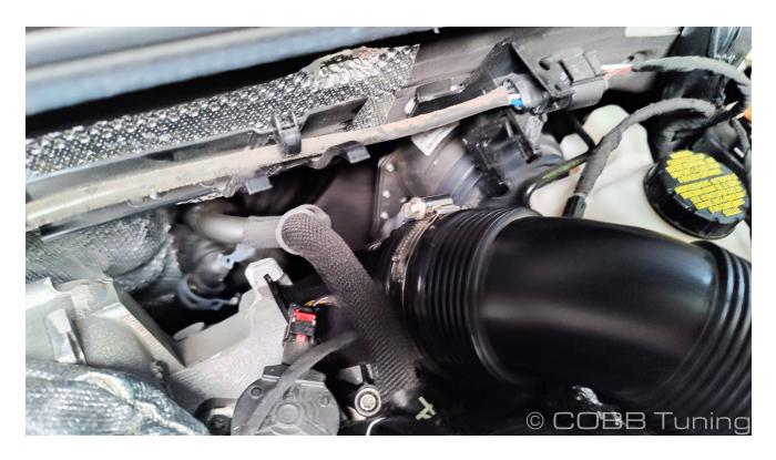
4. Take a T20 Torx screwdriver and remove the screws holding the stock snorkel in place.
