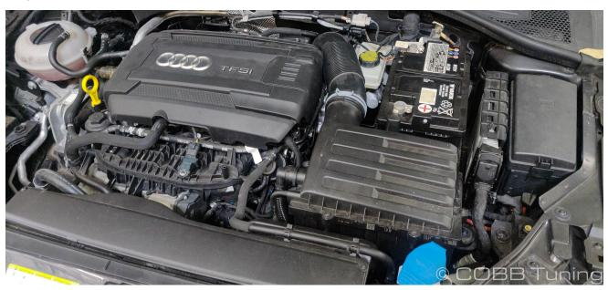
3. Using the hose clamp pliers, take off the clamp holding the stock intake tube to the turbo. Then pull the tube off of the turbo inlet housing.
