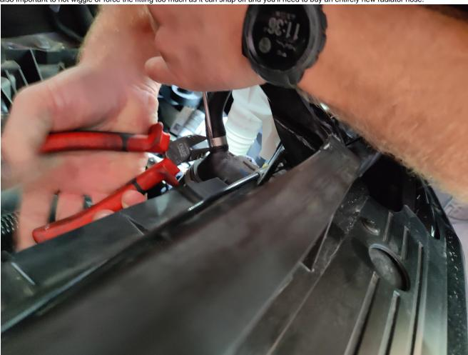
4. We recommend removing the line from the engine side first, as this allows a bit more room to catch the spills from the hose and metal tube. Remove the clamp with pliers and pull the hose off the line.
