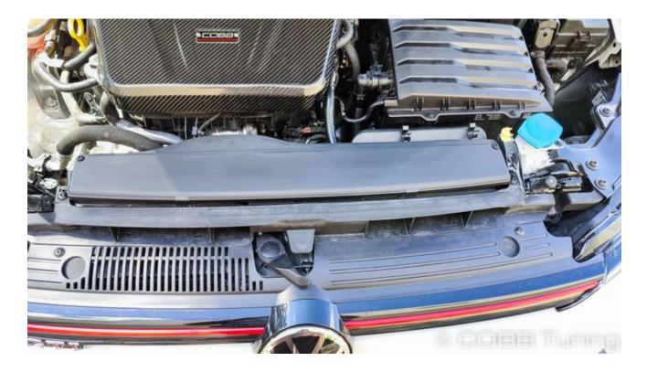
3. Next up we'll to take off the clamp holding the stock intake tube to the turboUsing your m7 nut driver or a phillips screwdriver, loosen the clamp. Then pull the tube off of the turbo inlet housing.
