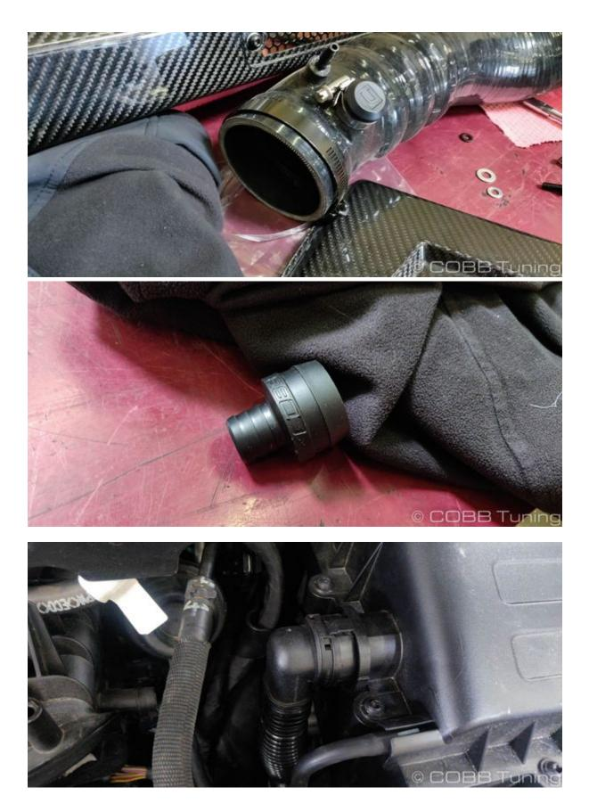
9. Add the provided small vacuum line to the small barbed fitting on the bottom of the intake silicone.
