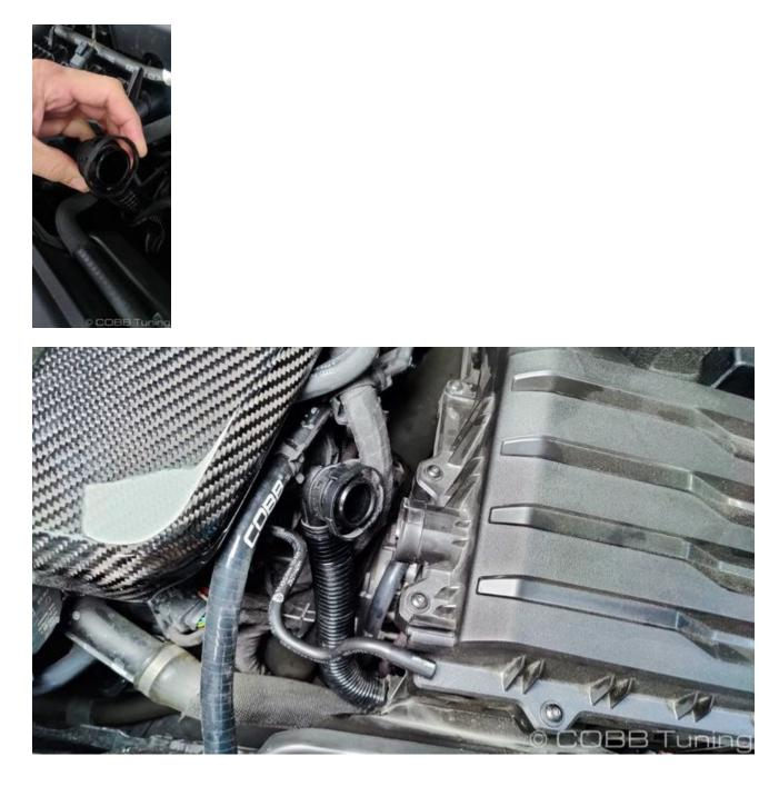
6. Now you should be able to pull the stock airbox and intake tube out of the car by popping the box off of the grommets that hold it in place. Lifting up in the back where the hose attaches the airbox and then rolling it towards you and out helps it drop out of the inlet box.
