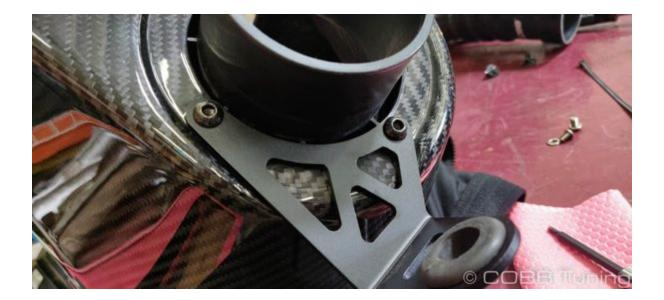
3. Pick up two more of the short bolts and add a washer to each. They can then be installed in the remaining two holes on the airbox.
