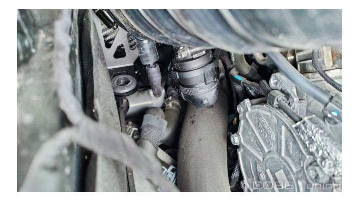
4. Connect the vacuum line from the intake silicon to the fitting where the factory vacuum line was connected.
