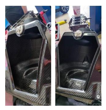
6. Carefully install the air filter into the airbox and around the mounting plate. It is a tight fit as the air filter is mostly retained in place by the airbox itself and the hose clamp is only a secondary connection, make sure as you install you don't crush the filter. Spin the hose clamp around to an angle you'll be able to reach before tightening it down with your 8mm socket or screwdriver.
