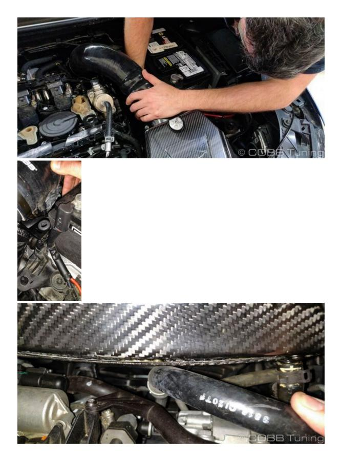
3. Connect the air pump (if equipped) to the bottom of the intake. You may need to carefully rotate the fitting in the tube, while doing so make sure to support the hose as you turn to avoid just twisting the tube itself.
