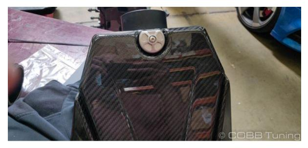
8. Install the small vacuum fitting to the reinforced silicon intake tube. If your vehicle has the factory air pump you'll install the adapter fitting. In our case our vehicle was not equipped with that so we installed the plug and secured it with the provided small hoseclamp.
