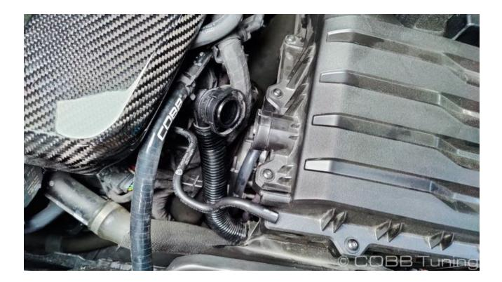
5. Unclip the air pump from the stock airbox.
