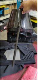
11. Slip clamps over both ends of the intake tube and then loosely slip it onto the airbox with the side with both fittings towards the airbox.
