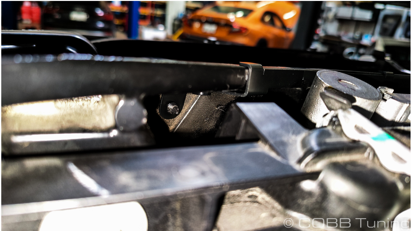
3. The threads should now line up with the two holes in the core support, with the tabs on the back holding it onto the core support.
