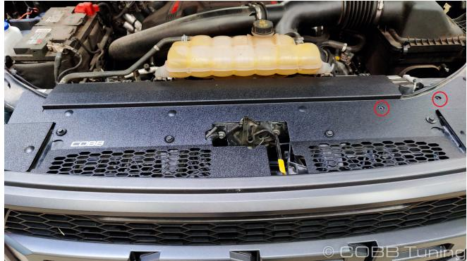
6. If you have the coolant reservoir and experience any rattling between the pieces, you can use the remaining portion of the edge trim around the center of the coolant tank and that should relieve any contact. However most vehicles should have a clear amount of space between the two.
