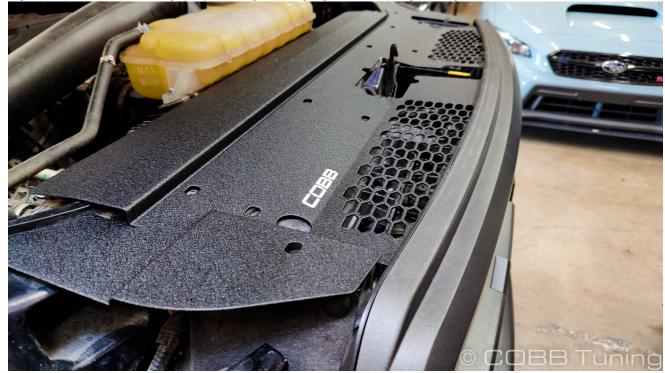
4. Loosely install the original bolts along the 4 center threaded bolt holes
