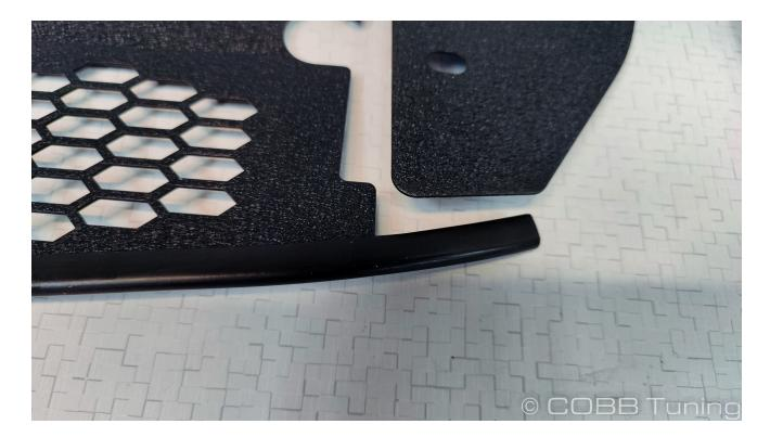
3. Slight it into place with the front edge you put the edge trim on going under the top edge of the grille.
