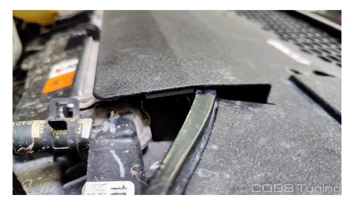
2. Line up the edge trim on the leading edge of the shroud (with the vents on it). Press it on starting at one end and trim it to fit at the other end.
