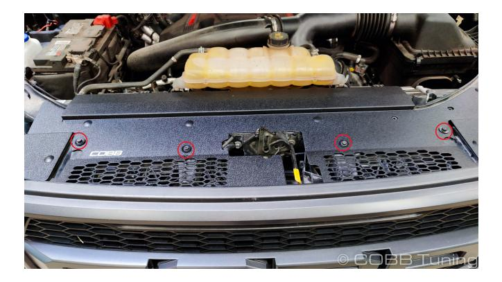
5. Add the supplied christmas tree clips in the 6 holes leaving the two marked in the picture empty (These are for the scoop).
