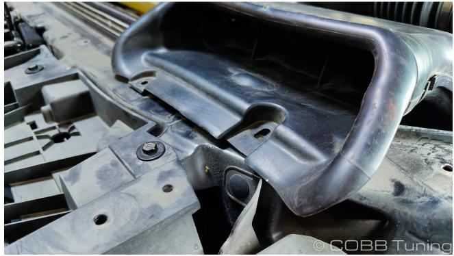
4. Grab your 8mm socket or wrench and remove the small bolt holding the intake scoop to the intake, then the snorkel can be removed from the engine bay.
