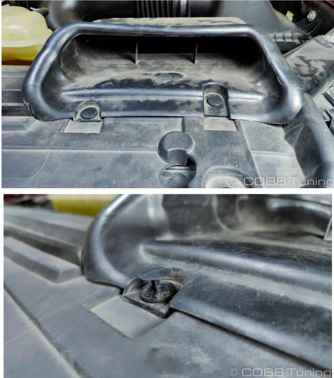
3. Remove the other trim clips that hold the plastic cover over the upper grill area. That cover can then be removed.
