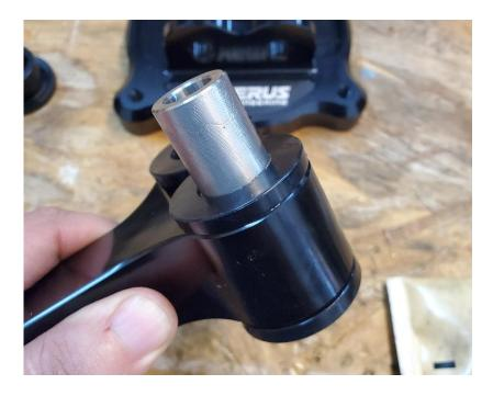
**2.12.4.** Push the bushing retainer into the base, and assemble the engine mount using the M12 bolts and nyloc nuts. Torque to 60 ft-lbs. Note: a dab of Loctite for extra security does not hurt either.
