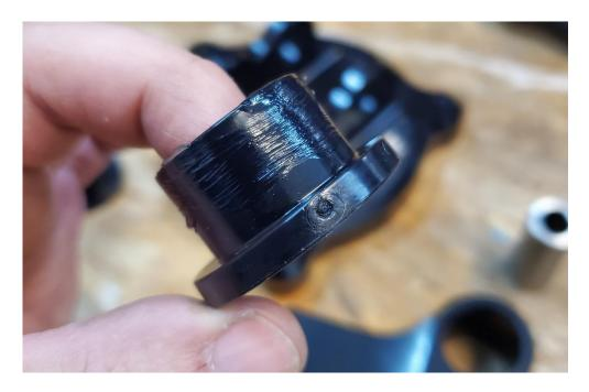
**2.12.3.** Press the bushings into the bushing retainer followed by the bolt sleeve.
