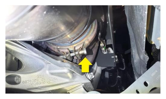
**2.6.2.** Remove two 13mm downpipe bracket nuts.
