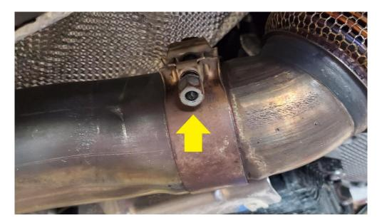
**2.6.5.** Remove the visible bolts for the chassis brace. This will allow the exhaust to hang down slightly.
