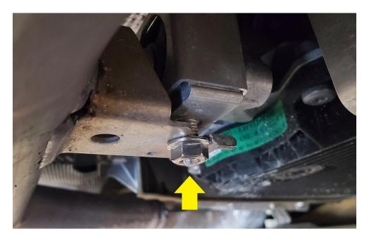
**2.6.4.** Loosen the rear exhaust clamp connection for the downpipe.
