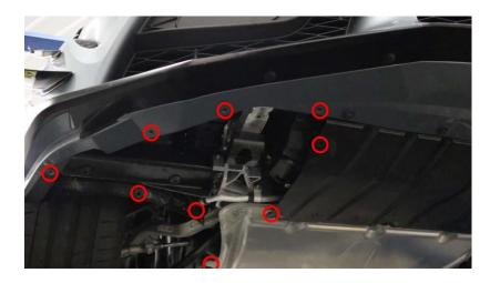
**2.6.** We also need to remove the (3) 16mm bolts circled in blue below.
