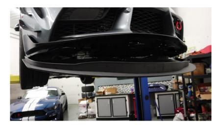
**5.3.** Now it is time to pivot the splitter up and check how well our brackets line up with the mounting holes in the splitter. Again, the splitter brackets need to be loosely installed so that they can be moved a small amount for test fitting.
