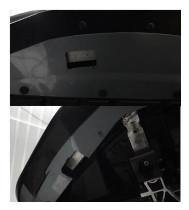
**3.5.** Starting with the two centermost locations, we need to grab the correct small brackets to mark our holes for drilling. These brackets only have two slots, whereas the outside brackets will have an additional square cut-out in the center.
