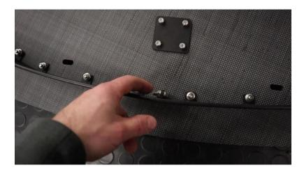
**4.11.** Loosely install the air dam onto the splitter using the 20mm long BHCS and 18mm fender washers on the bottom side and then a serrated nut on the top side. Only install the nuts hand tight initially. Once the splitter is on car, we can make final adjustments for the air dam before fully tightening it down. Below is what the splitter should look like before getting installed on car.
