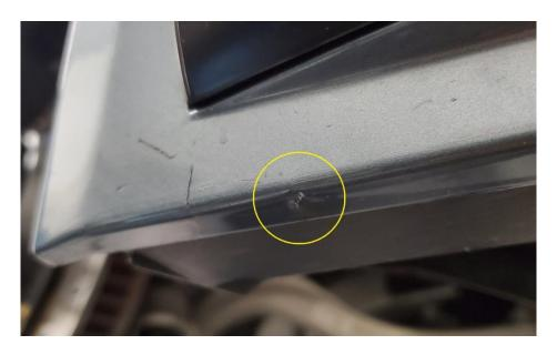
**5.10.** Using the mark(s) as a reference, use a 1/2" drill bit and drill the mark out so the hardware can sit inside of it when the bumper is completely installed.
