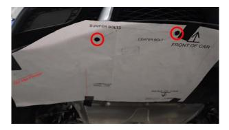
**3.2.** Once the templates are correctly placed, use a 3/8" drill bit to drill starter holes for bumper trimming.
