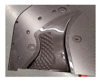
**4.4.** With the diffuser lined up correctly, scribe the holes that need to be drilled by using a small pick through the pre-drilled holes in the splitter.
