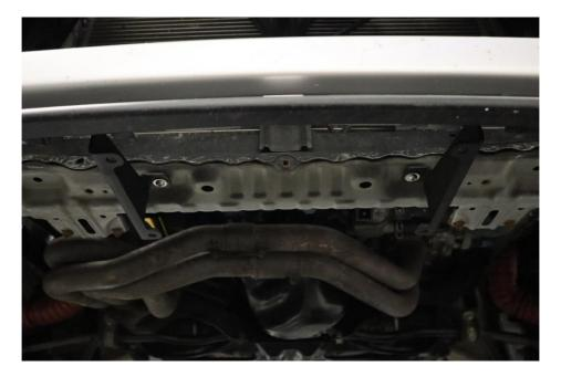
**2.5.1.** Next, we will install the outer mounting brackets in the orientation shown below. Use two 12mm long M6 x 1.0 BHCS with two 18mm M6 fender washers. These brackets should be "pointing" straight towards the rear of the car.
