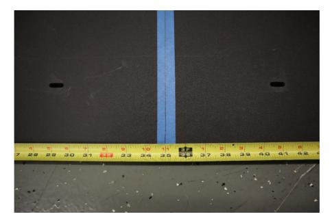
**3.2.** Next, place tape down on the splitter silhouetting or "outlining" the bumper profile as shown below.
