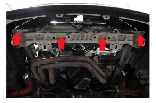
**2.4.** Locate the four mounting locations for the splitter mounting brackets.
