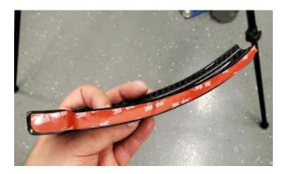
2.9. Check fitment of the dive planes to the bumper before final install. The dive planes should fit the bumper perfectly. If they do not, ensure the template is installed correctly and adjust as necessary. Pay special attention to how the dive plane wraps around the "fang" which is pointed out by arrows below.
