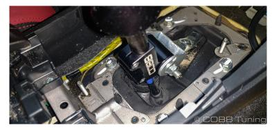
23. Reinstall the center console shifter surround trim piece making sure to reattach the wiring harness for the lighter and screw the shift knob back into place making sure it is tight. Make sure the shift boot is reattached around the trim piece.
