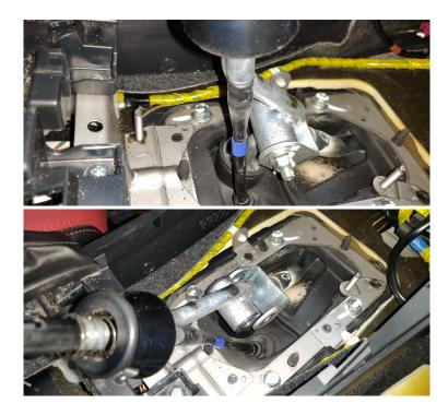
11. Next, using snap ring pliers remove the c-clip that holds the bottom cup in.
