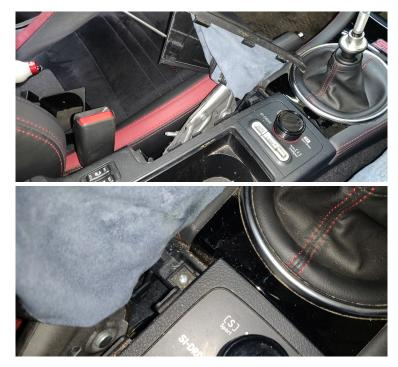
6. (08+ STi Only) Lift up on the rear of the shifter surround and slide it back towards the rear of the car. Unclip the wire underneath this piece in order to be able to set the trim piece aside.
