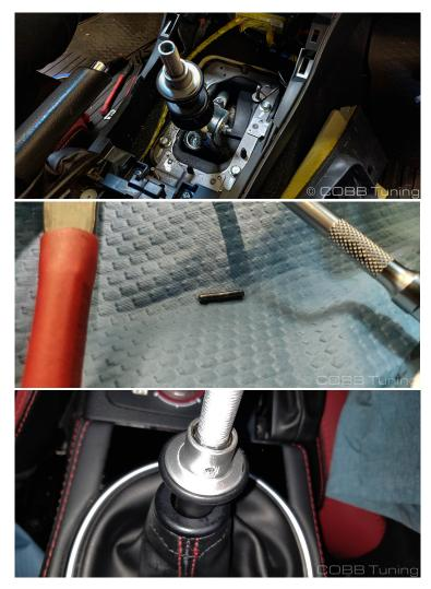
10. Use (2) 12mm boxed end wrenches, one on either side, to remove the bolt that holds the shift lever to the shift linkage as shown in the picture below. DO NOT misplace the nut and bolt, as they will be reused with the COBB Tuning Short Shifter.
