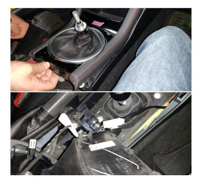
7. Unscrew the two plastic clips using a flat blade screwdriver and remove the shift boot bellows
