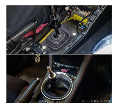
24. Congratulations and enjoy your shifting with your new COBB Tuning 6-Speed Double Adjustable Short Throw Shifter. Future adjustments can be made very easily by just removing the center console shifter surround trim piece as the clamp screws are easily accessible.
