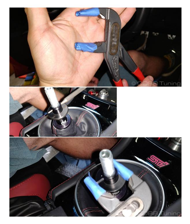
20. Sometimes as you tap the pin into place it can push the reverse lockout cable up against the side of the shifter. To avoid this happening, tap the pin slightly too far, then tap it back the other way to even it out back into the middle.
