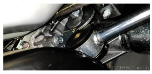
3. Slip the bushing back over the stud (5-speed cars) or add the bolt back into the bushing.
