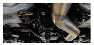
4. Loosen the four 14mm bolts on the rear lateral (side to side) transmission mount.
