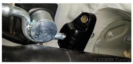
4. Using the provided bolts install the rear bushing using a 12mm socket tighten to 13.3 ft-lbs (18Nm)
