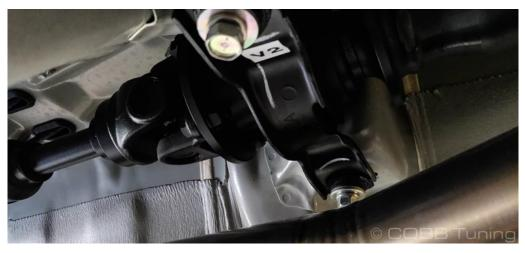
8. Using your 12mm socket and ratchet, remove the two bolts holding the rear shifter bushing in place.
