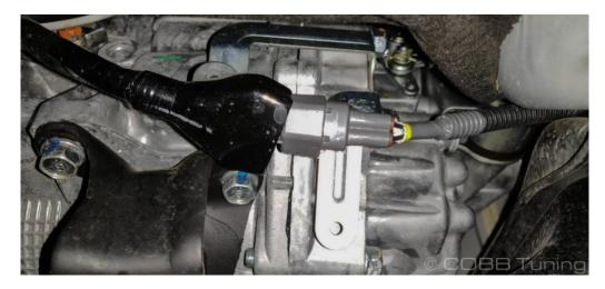
4. Using a 22mm oxygen sensor wrench remove your rear o2 sensor and set it somewhere safe.
